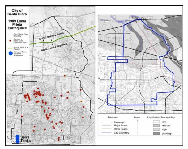
Figure 10. 1989 Loma Prieta Earthquake - Locations of Pipe Damage in Santa Clara
