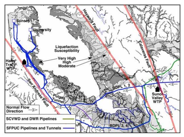
Figure 1. SFPUC Transmission System (2005) and Geologic Hazards (Knudson et al 2000)
