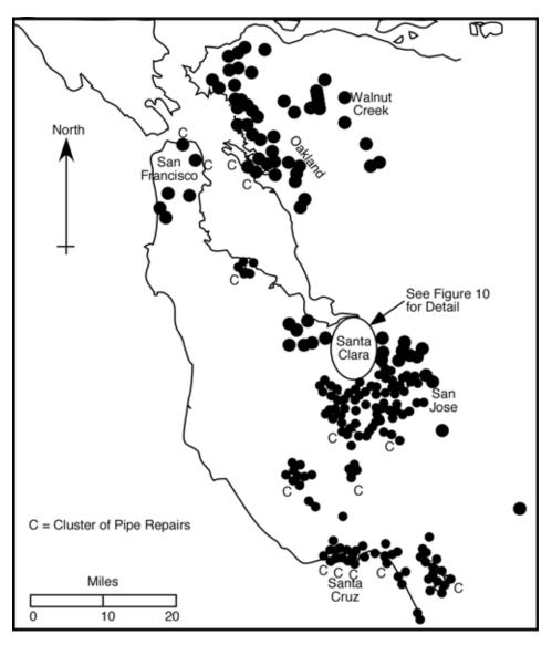
Figure 7. 1989 Loma Prieta Earthquake – Locations of Pipe Damage
