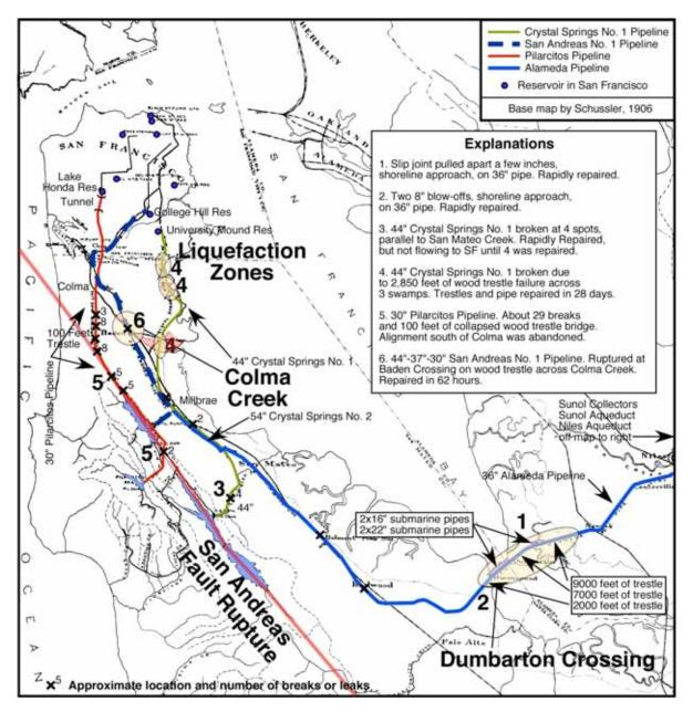
Figure 3. Damage to SFPUC (then SVWC) Transmission System, 1906 Earthquake
