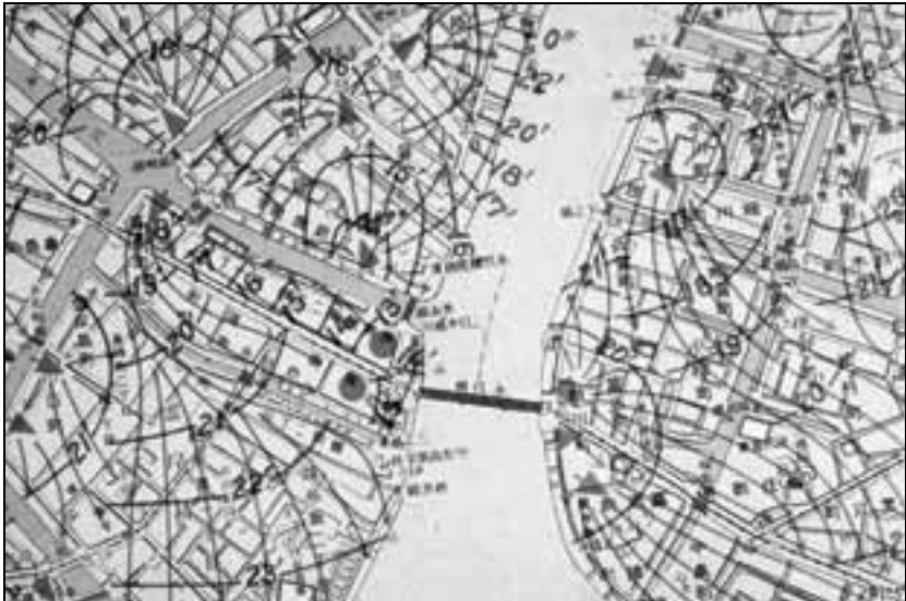
Figure 2-13 Firespread in Central Tokyo, showing direction and hourly progress of flame front
