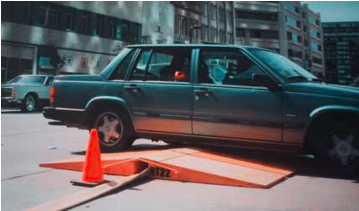
Figure 13-8. Use of Ramp Over A 5" Diameter Flex Hose
