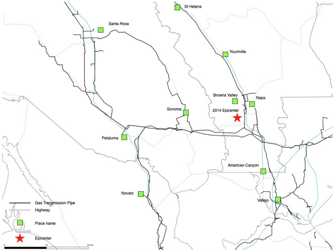
Figure 6.17-1. Gas System near Napa
