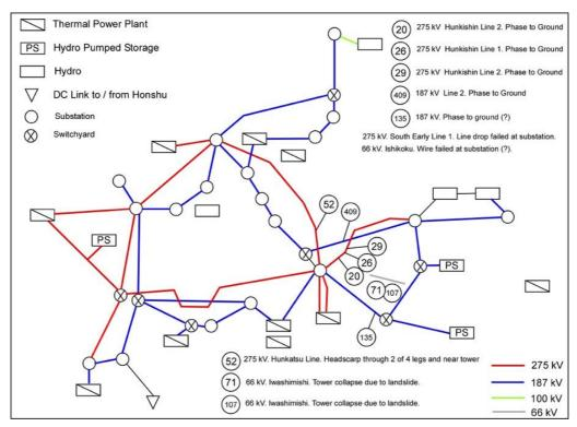
Fig. 7. Locations of Transmission Tower Damage
