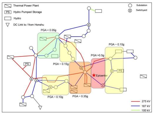
Fig. 6. Shaking Levels in the Transmission Grid
