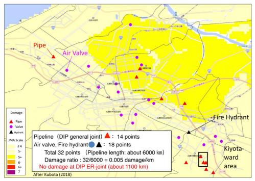
Fig. 9. Location of Water Pipeline Damage
