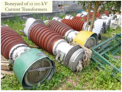
Figure 4-7. 110 kV Broken Current Transformers
