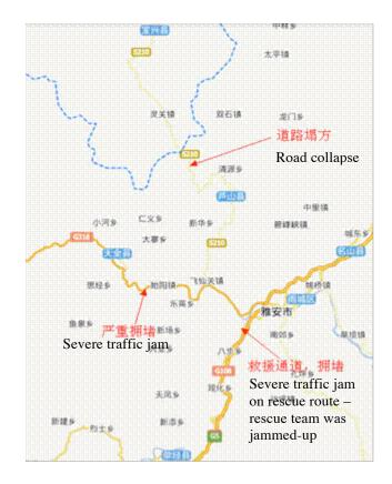
Figure 7-2. Map of roads and highways in Lushan earthquake damage area, some areas of severe problems noted for G318, G108, and S210
