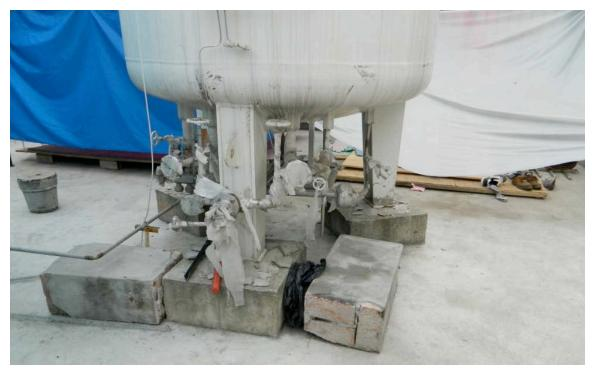
Figure 12-3. Unanchored Liquid Oxygen tank rocked at the hospital in Lushan. The rocking resulted in failure of the attached pipe. All liquid oxygen evaporated.
