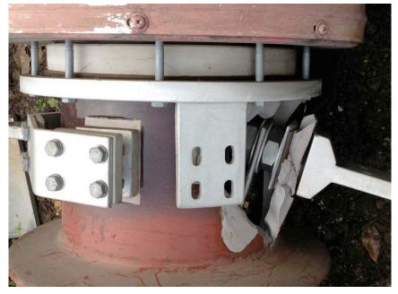
Figure 4-8. 110 kV Broken Current Transformers
