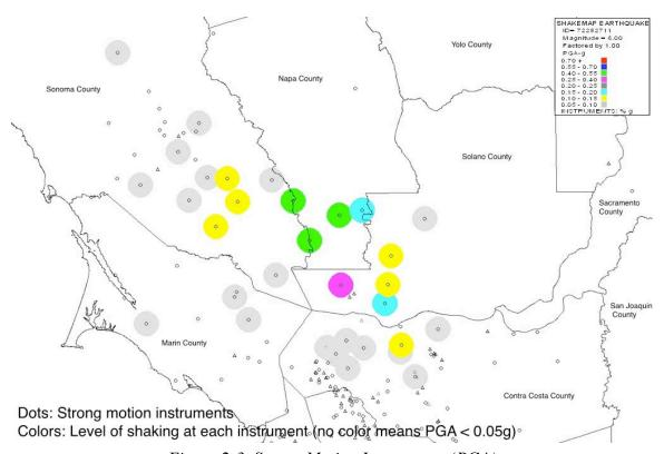
Figure 2-3. Strong Motion Instruments (PGA)
