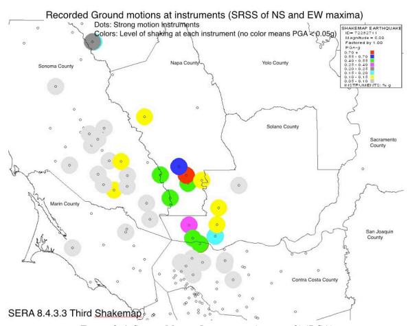
Figure 2-4. Strong Motion Instruments (version 3) (PGA)
