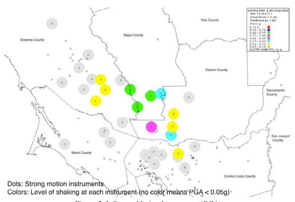
Figure 2-3. Strong Motion Instruments (PGA)
