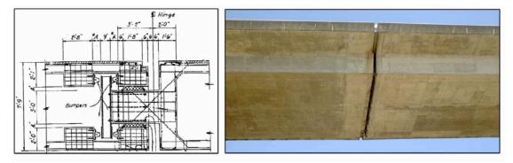
Figure 5-12. Unusual in-span hinges on the Napa River BOH
