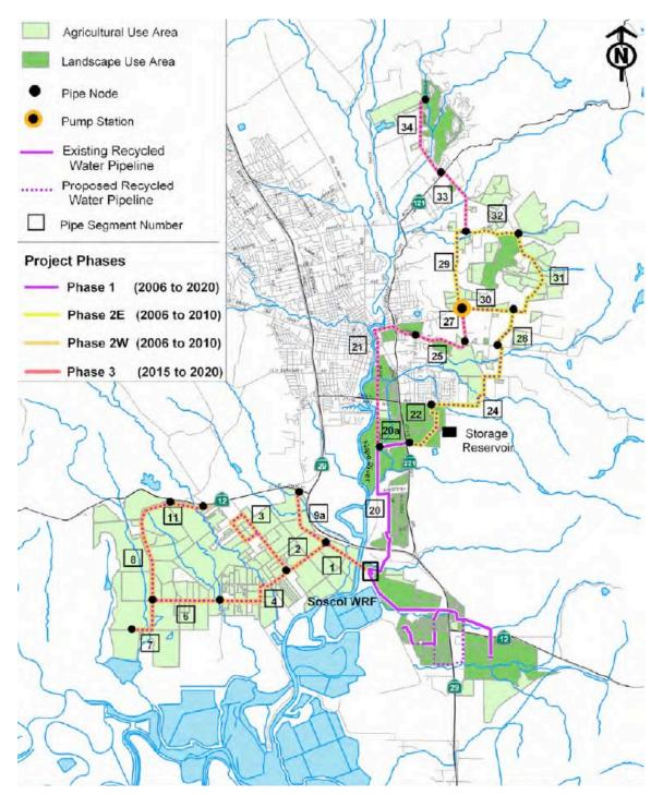
Figure 4-17. Napa Recycled Water System
