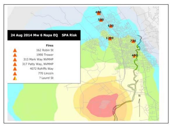
Figure 7-1. Location of Fires in Napa, with Overlay of ShakeMap (v1)
