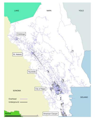
Fig. 2 - Overhead and Underground Distribution Lines in Napa County
