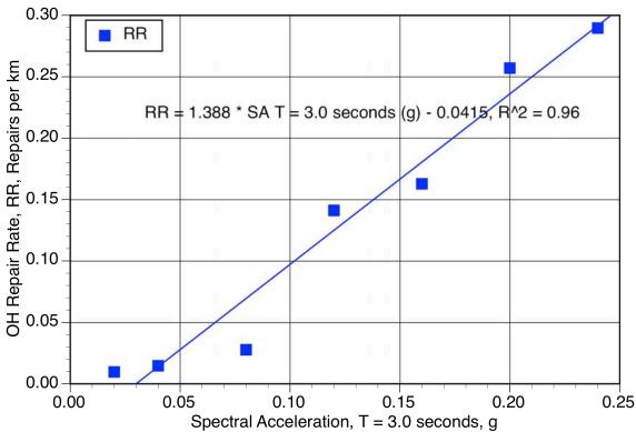
Fig. 7 - Repair Rate, Overheads, Using PSA (T = 3.0 seconds)
