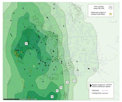
Fig. 5 - Electric Distribution System Repairs near the City of Napa
