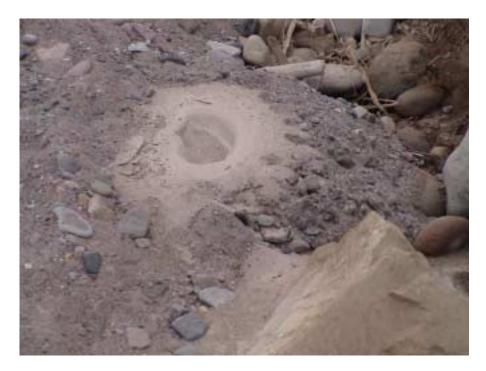
Figure 3-2. Sand Boil in river bed. The boil measures about 6 inches in diameter.
