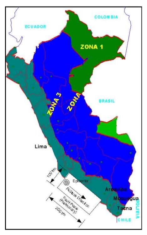
Figure 2-3. Map of Peru Showing Seismic Zones and Rupture Fault Plane
