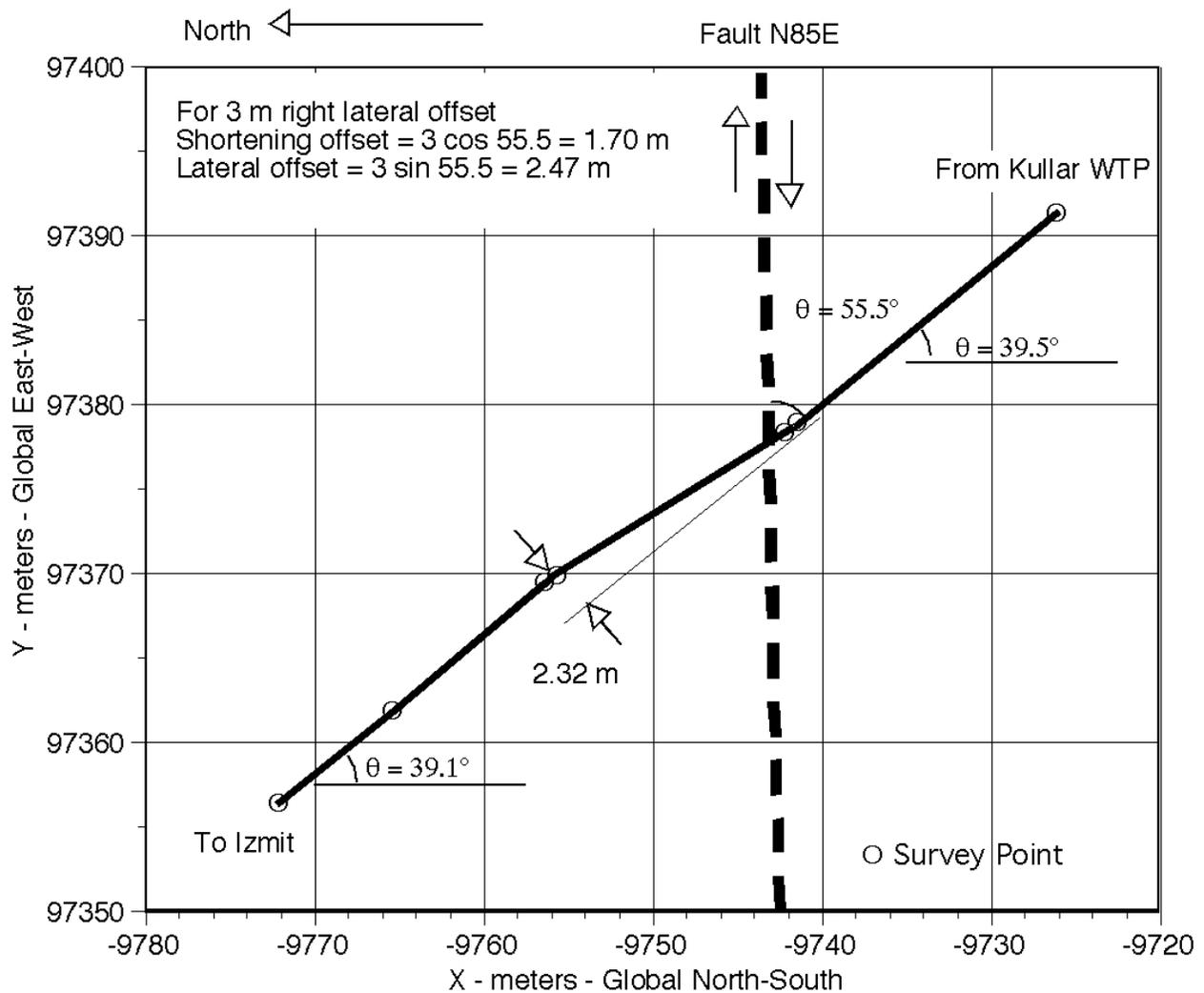
Figure 5. Pipeline and Fault Geometry
