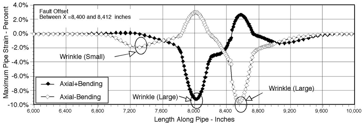
Figure 7. Variation of Strain along the Pipeline Near the Fault, Model 4
