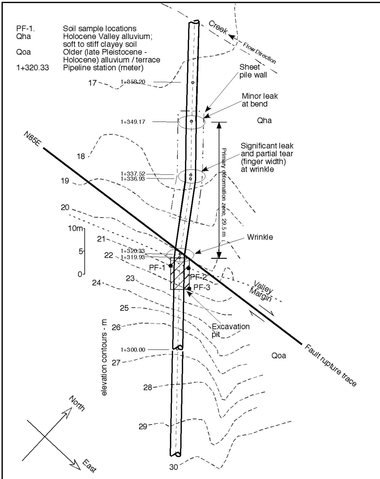
Figure 4. Pipeline and Fault Location After Earthquake.
