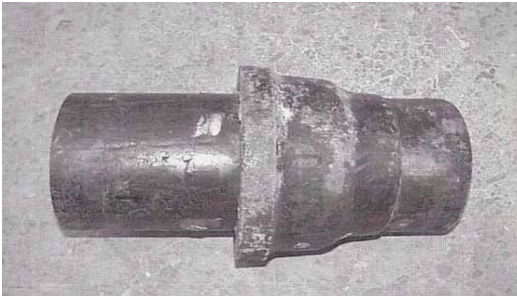
Figure 10-1. Cast Iron Pipe – Bell and Spigot Joint
