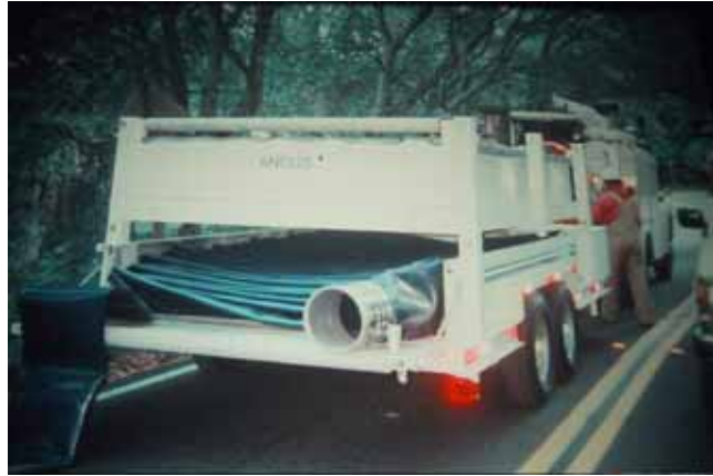
Figure 9-4. Deployment Using Flaking Box
