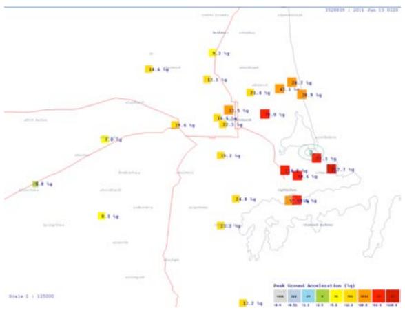
Figure 2-20. Recorded Ground Motions (PGA), June 13 2011
