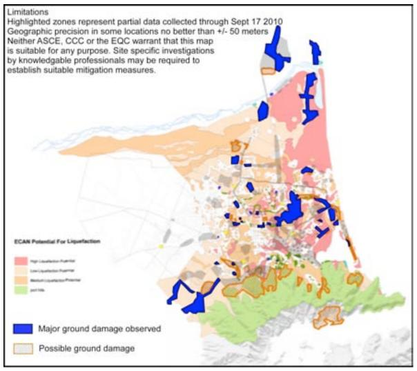
Figure 2-34. Map Showing Observed Major (Blue) or Possible (Diagonal) Ground Deformation
