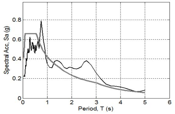
Figure 2-13. Horizontal Response Spectra (5% Damping), Design (smooth) and Recorded
