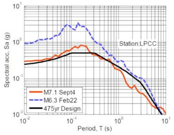
Figure 2-17. Comparison of Response Spectra between February 2011and September 2010 Earthquakes (source Brendon Bradley, GNS). Rock site, Port of Lyttleton.
