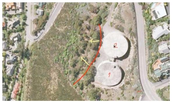
Figure 6-21. Landslide Scarp, McCormacks Bay Tank Site
