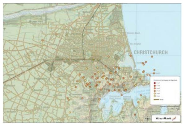
Figure 12-22. Aftershock Sequence with Respect to KiwiRail Lines
