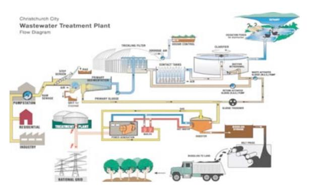
Figure 7-38. Process Flow Diagram, Bromley WWTP
