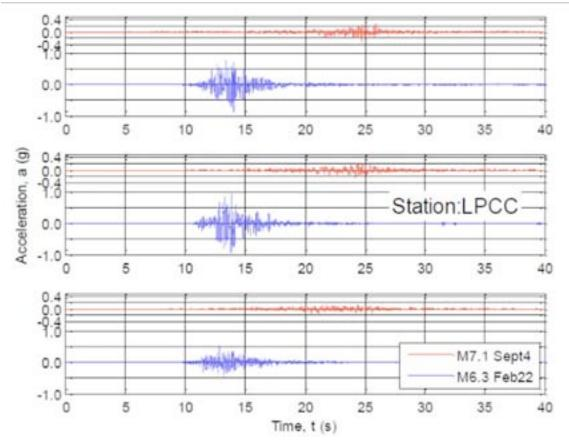
Figure 2-18. Comparison of Response Spectra and acceleration time history recordings between February 2011 and September 2010 Earthquakes (source Brendon Bradley, GNS)
