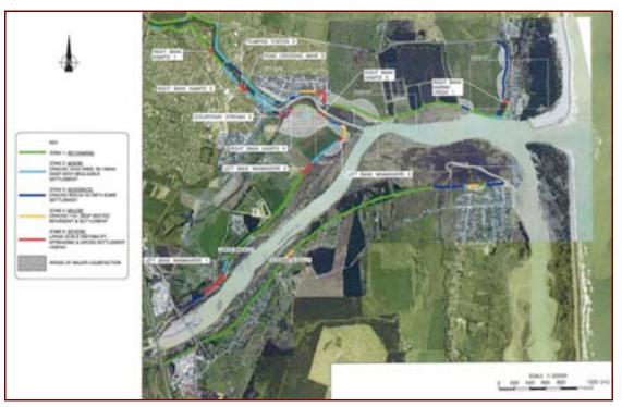
Figure 14-1. Stopbank damage surveyed by Riley Consultants
