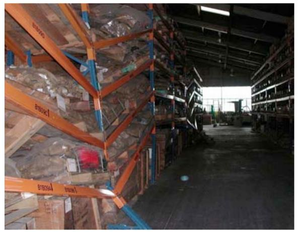
Figure 17-1. Damaged Storage Rack, Addington Warehouse
