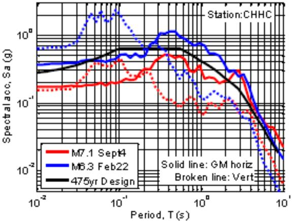
Figure 2-16. Comparison of Response Spectra between February 2011 and September 2010 Earthquakes (source Brendon Bradley, GNS). Soil site, Christchurch Hospital.
