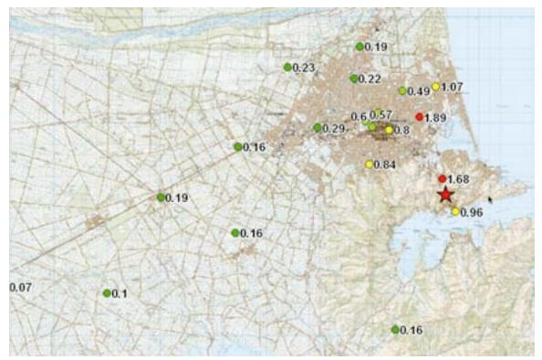
Figure 2-11. Recorded Ground Motions (PGA), Feb 22 2011
