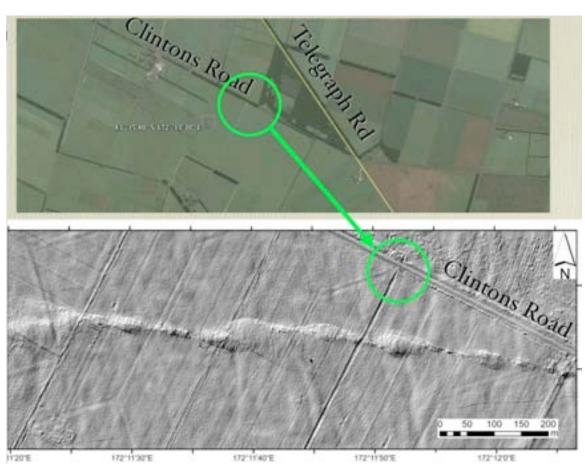
Figure 2-31. Location Map (Upper) and Lidar Map of Fault Offset Zone (Lower)
