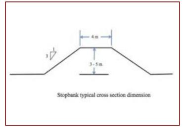
Figure 14-2. Stopbank Cross Section
