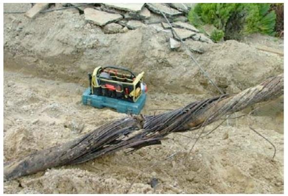
Figure 4-58. Damaged Buried Cable– Sept 4 2010 – Mainpower
