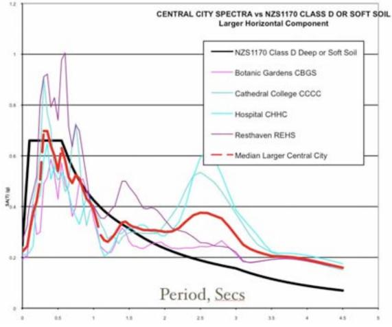
Figure 2-14. Central City Horizontal Spectra vs. NZS 1170 Class D or Soft Soil
