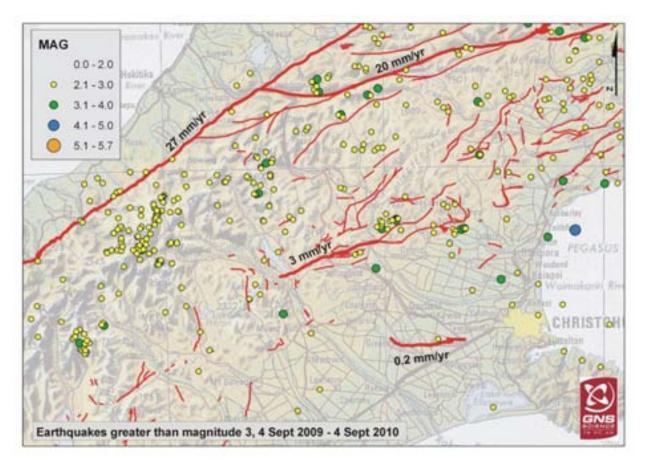
Figure 2-2. Map of Canterbury Area with Slip Rates of Selected Faults and Earthquake Epicenters, 2009-2010
