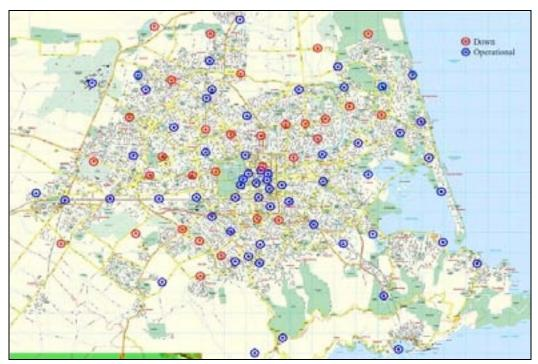
Figure 5-3. Locations of BTS out of power (Courtesy of Vodafone New Zealand)
