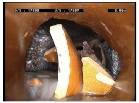
Figure 7-10. CCTV picture of Broken Sewer, WDC
