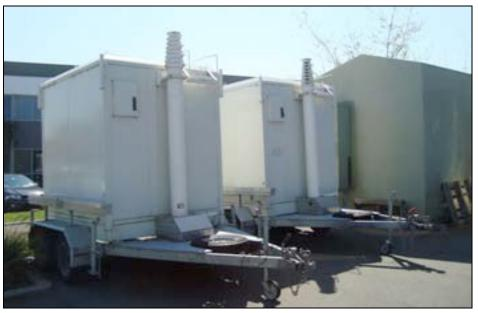
Figure 5-5. Vodafone Cellsite On Wheels (COW).
