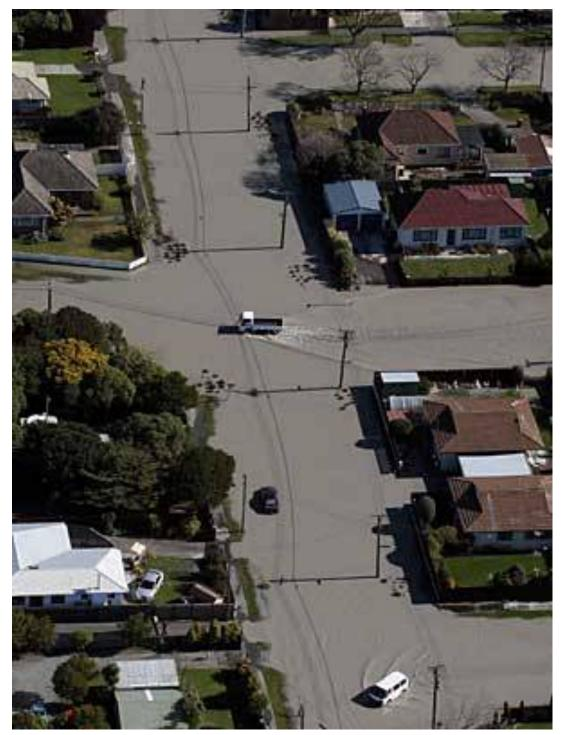
Figure 2-33. Flooding due to Liquefaction
