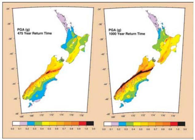
Figure 3-1. Seismic Hazard Map for New Zealand, Horizontal PGA (g)
