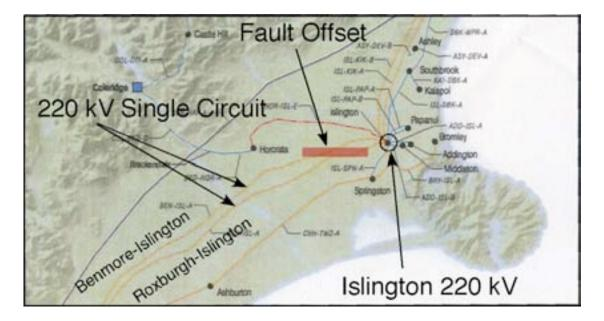
Figure 4-1. Transpower Regional High Voltage Grid (Red line shows approximate location of faulting for the Sept 2010 event)
