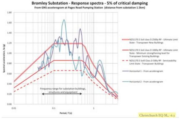
Figure 4-23. Horizontal Response Spectra (5% Damping) Near Bromley Substation
