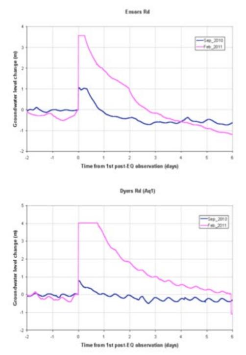
Figure 6-36. Change in Groundwater Level After Sept 2010 and Feb 2011 Earthquakes
