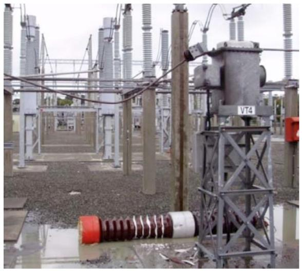
Figure 4-30. Broken Voltage Transformer, 220 kV, Bromley Substation
