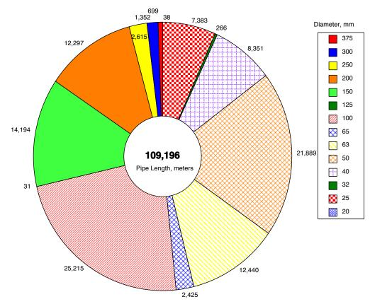
Figure 6-16. Length of Water Pipe, by Diameter (mm), Kaiapoi
