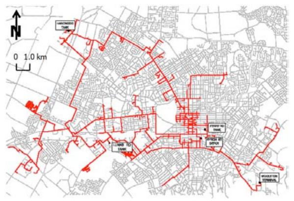
Figure 8-1. Contact Energy Gas Service Areas and Pipeline Network in Christchurch
