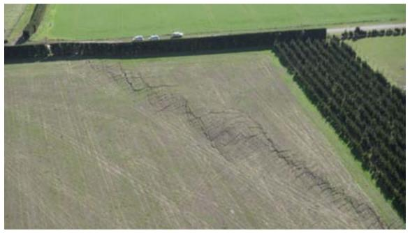
Figure 2-30. Right Lateral Fault with En-Echelon Cracks
