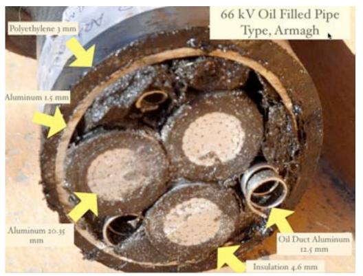
Figure 4-53. Cross Section of 66 kV Buried Oil-Filled Cable
