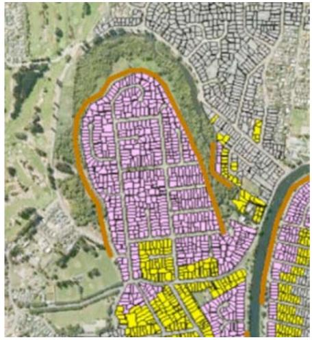
Figure 6-31. Horseshoe Lake Liquefaction, September 2010
