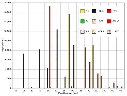
Figure 6-15. Length of Water Pipe, by Pipe Type, Kaiapoi
