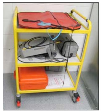
Figure 5-15. The cart shown was not secured to wall or to the floor. The wheels may be locked but the cart can topple or the equipment on it may fall.
