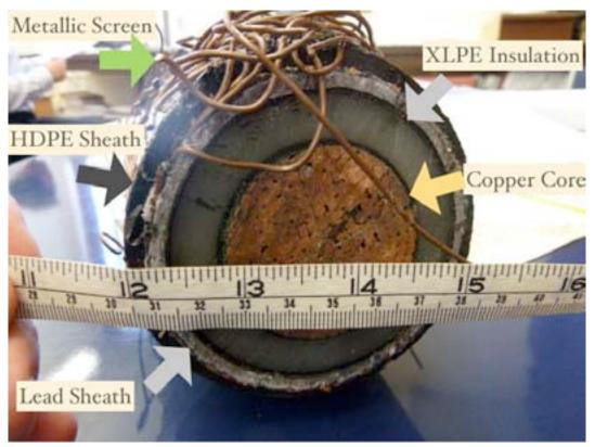
Figure 4-54. Cross Section of 66 kV Buried XLPE Cable (Scale is inches / cm)
