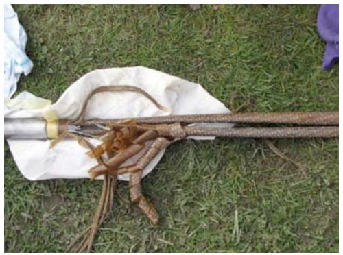
Figure 4-60. Damaged Distribution Cable – Kaiapoi – Sept 2010
