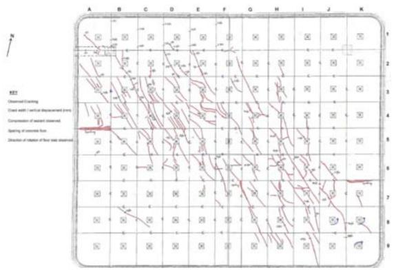
Figure 6-26. Interior Inspection of March 3 and 4, 2011
