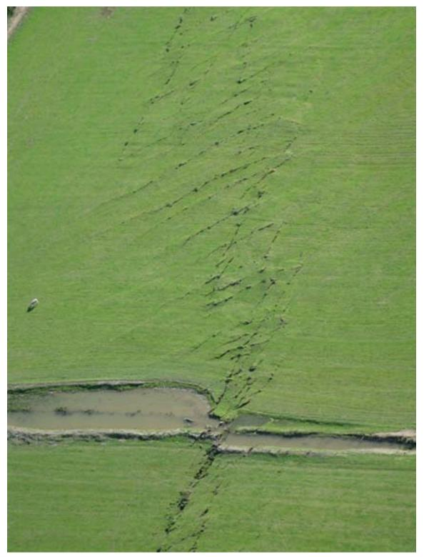
Figure 2-29. Right Lateral Fault with En-Echelon Cracks (Quigley, Univ. Canterbury)
