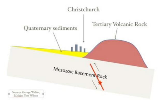
Figure 2-9. Cross section, February 22, 2011 Fault Rupture (Looking Northeast)
