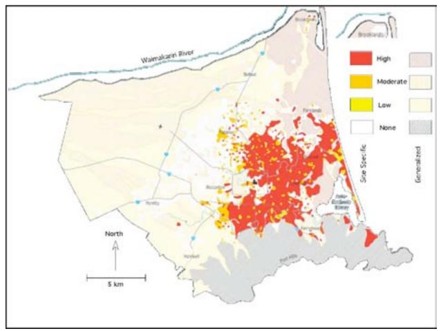
*Figure 2-32. Liquefaction Potential Hazard Map (adapted from Ecan, 2004)*
