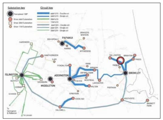
Figure 4-17. Orion System (Damage Location to 66 kV Circled, September 2010)
