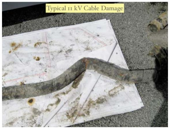
Figure 4-50. Failure of Typical 11 kV Buried Cable, Feb 22 2011
