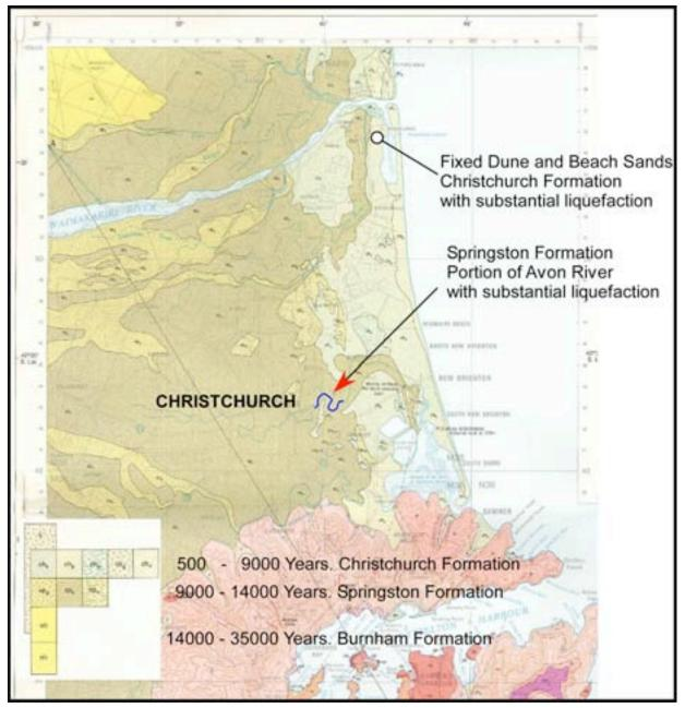
Figure 2-8. Regional Geologic Map (Adapted from Sewell et al, 1993)
