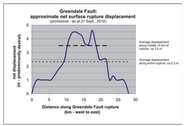
Figure 2-24. Measured Fault Offset
