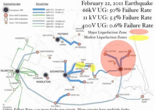
Fallure Rate: 1 or more faults per circuit. Many circuits have multiple faults
