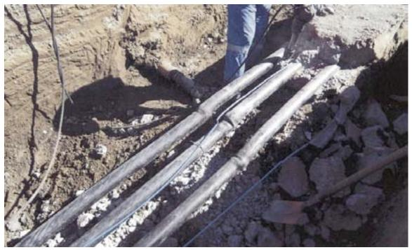
Figure 4-52. Failure of Three 66 kV Buried XLPE Cables, Feb 22 2011
