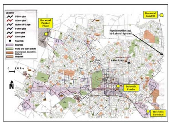
Figure 8-2. Contact Energy Gas Distribution Network with Road System and Cultural Features of Christchurch
