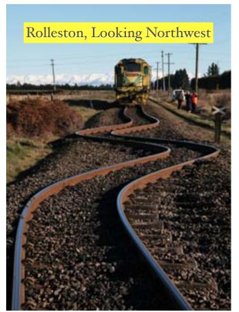
Figure 12-4. Buckling of Rails at Fault Offset Location (Baxter)
