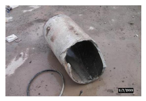
Figure 11. Damage to 14" Diameter AC Pipe – Liquefaction Area
