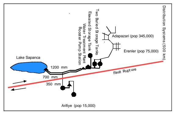
Figure 3. Water System Schematic Diagram for the Adapazari – Arifiye – Erenler Area
