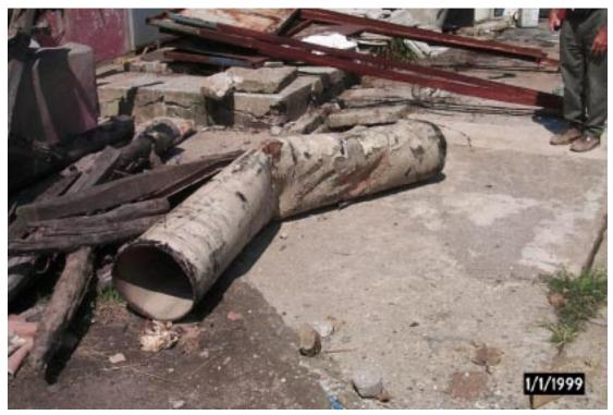
Figure 4. Ovalized Steel Pipeline, Removed From Fault Offset Location, Arifiye
