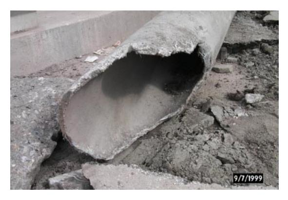
Figure 12. Common Damage Pattern to AC Pipe In Areas with Settlement
