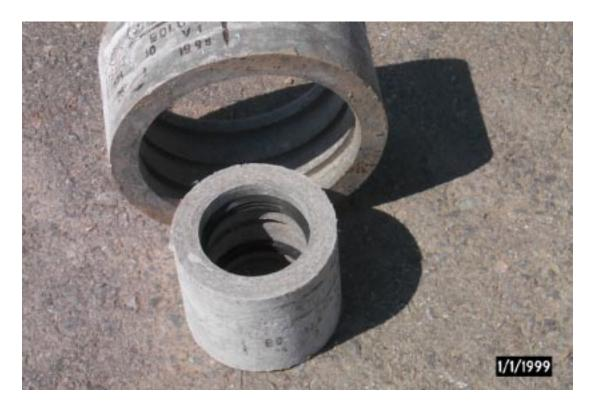
Figure 10. Typical Rubber Gasket Joint Fitting for AC Pipe, Common to All Water Systems in the Area
