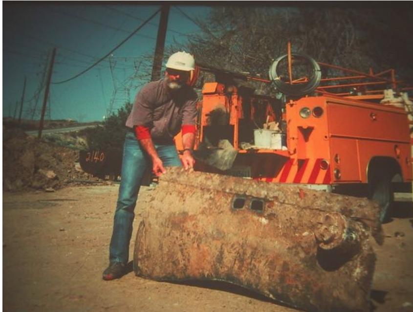
Figure 6-1. Tim Hall with Segment of Damaged LADWP Riveted Pipe, 1994
