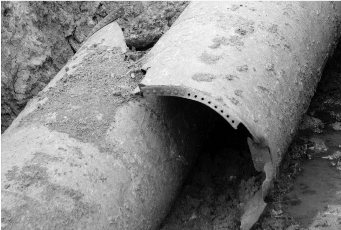
Figure 4.1.6-3. Closeup of Figure 4.1.6-2 showing rivets. (Photo Schussler HS6)
