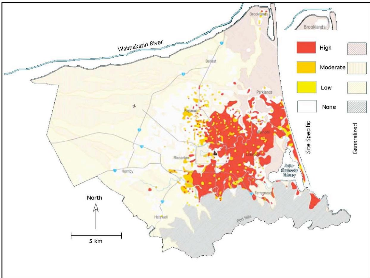
Figure 10. Liquefaction Potential Hazard Map (adapted from Ecan, 2004)
