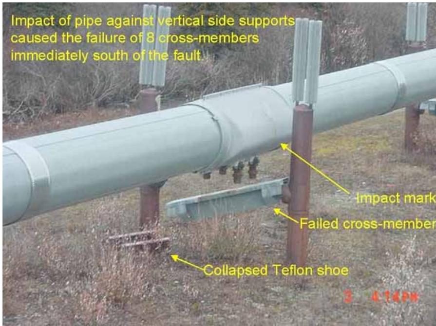
Figure 3.12. Damage to vertical and horizontal members and to teflon shoe supports (Alyeska)
