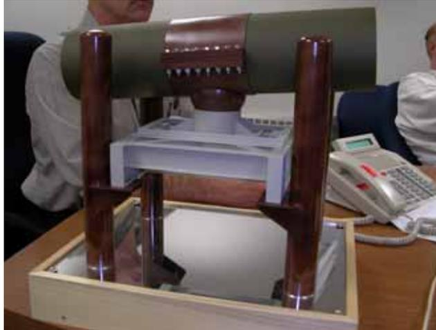
*Figure 3.4. Model of four-legged pipe support*
