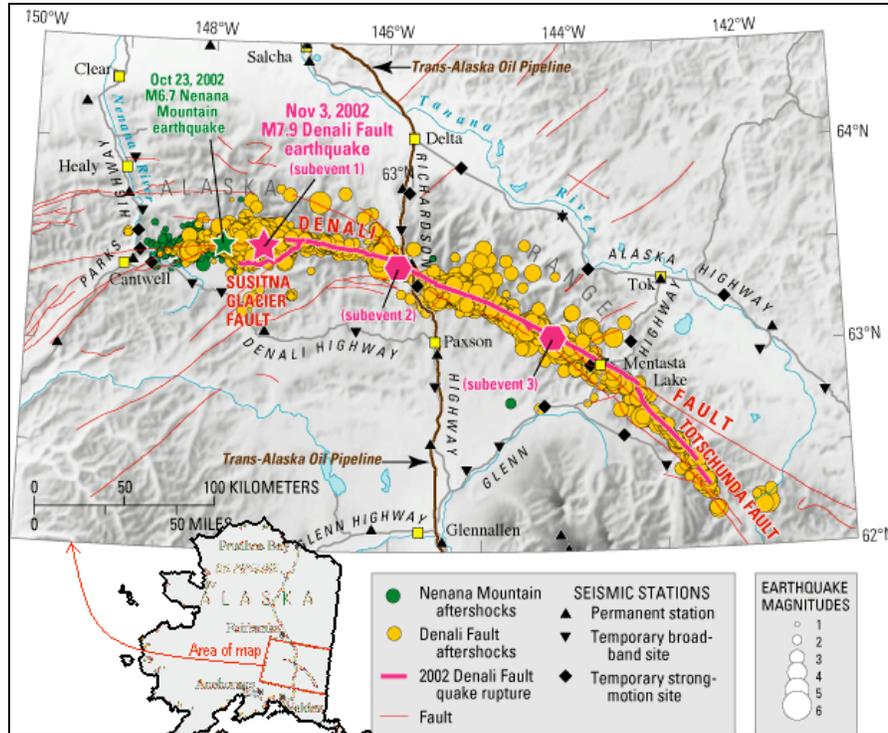
Figure 2.2. Map showing fault rupture and other significant features of two earthquakes (USGS)
