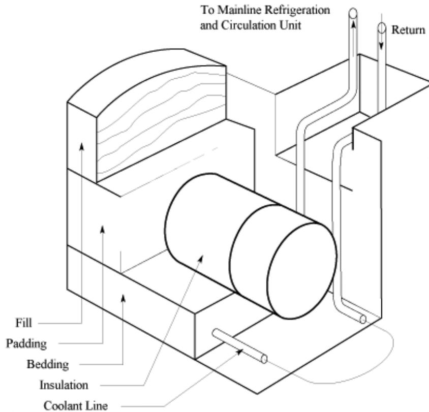
Figure 3.2. Special burial of Alyeska oil pipeline (Alyeska).
