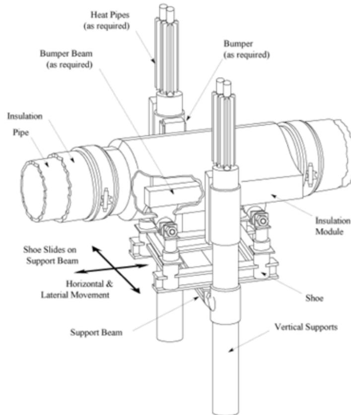
Figure 3.3. Two-legged pipe support (Alyeska)
