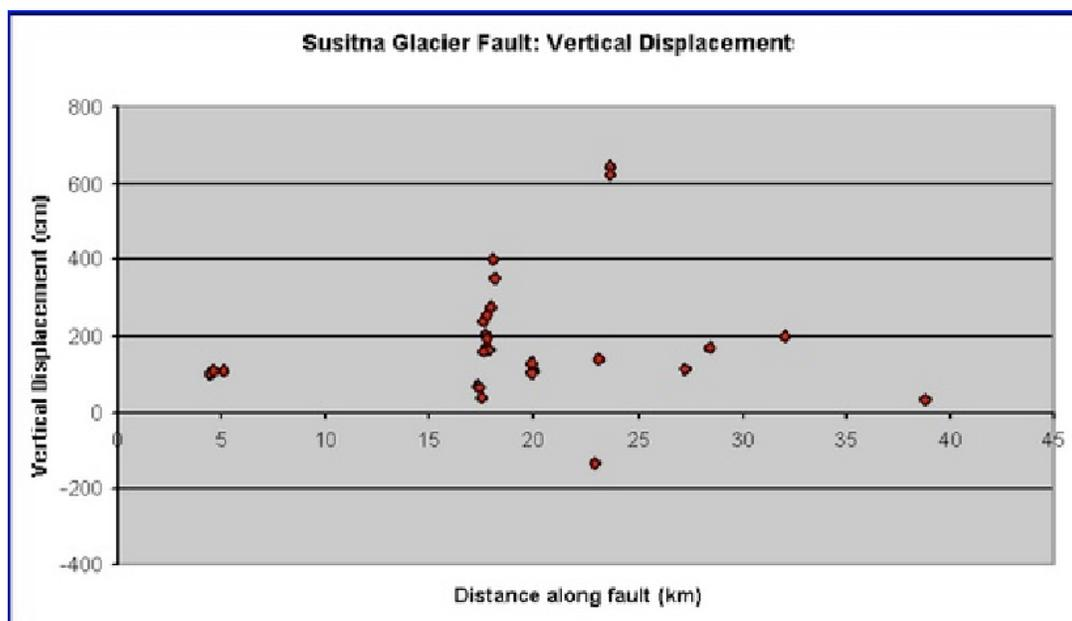
Figure 2.6. Vertical offset along the Susitna Glacier Fault (USGS)
