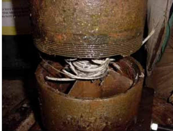
*Figure 4.1. Damaged well casing at Fort Richardson in Anchorage*
