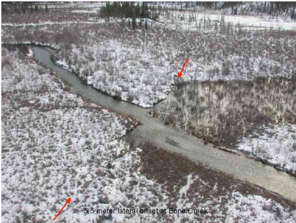
Figure 2.5. Lateral Offset along Denali Fault (USGS)
