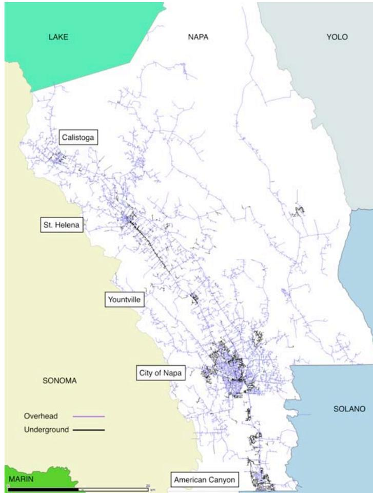
Figure 2. Overhead and Underground Distribution Lines in Napa County
