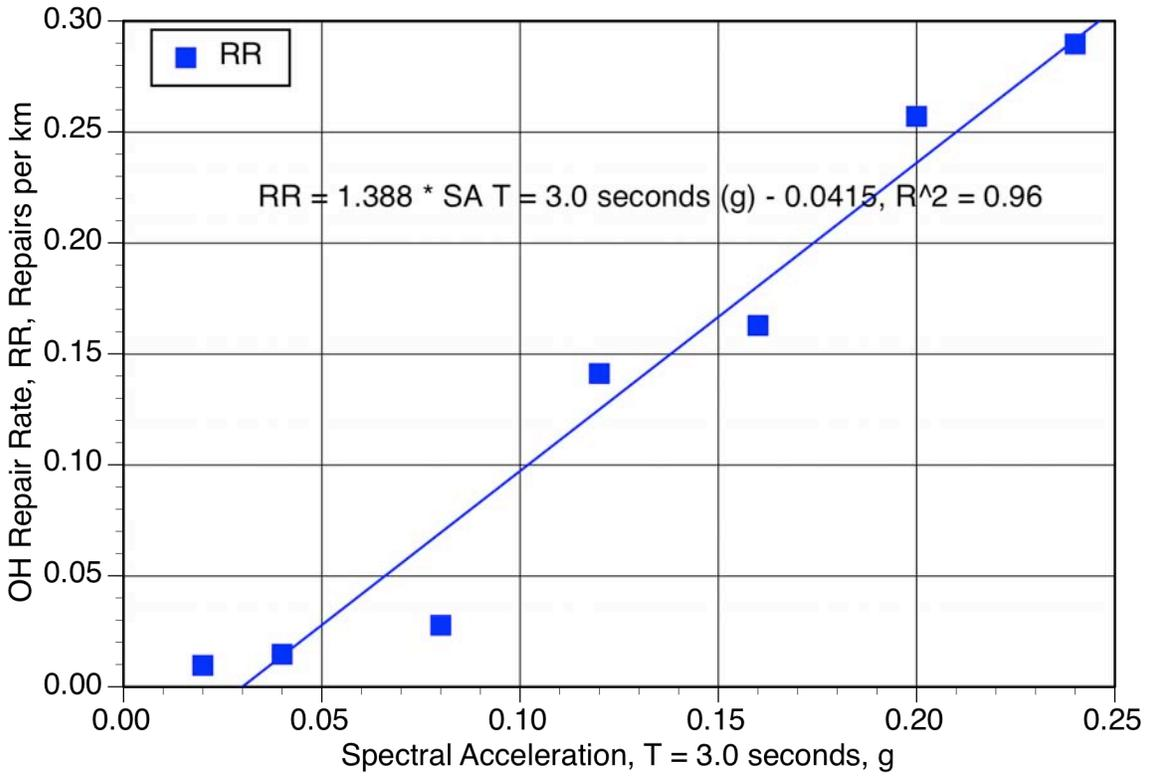
Figure 6. Repair Rate, Overheads, Using SA (T = 3.0 seconds)
