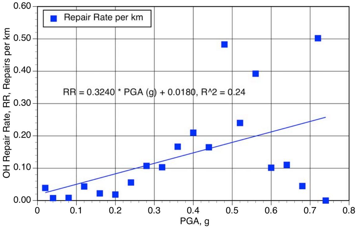
Figure 5. Repair Rate, Overheads, Using PGA
