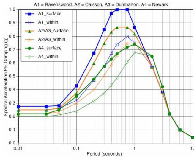
Figure 6. Horizontal Spectra, 125 Year Earthquake
