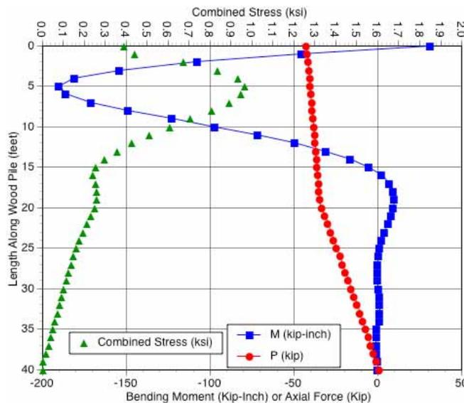
Figure 7. Pile Loads and Stress, Bent A Transverse Load of 30 Kips
