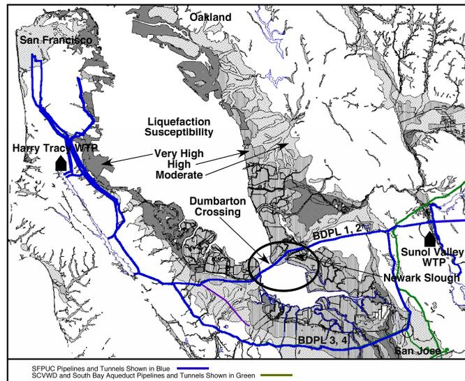
Figure 1. The Bay Division Pipelines 1 and 2 Crossing at Dumbarton
