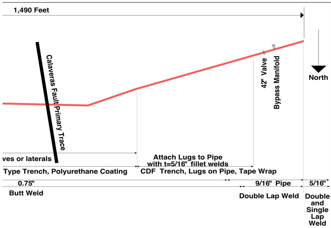
Figure 4b. Pipe Alignment With Main Design Features (West of Fault)
