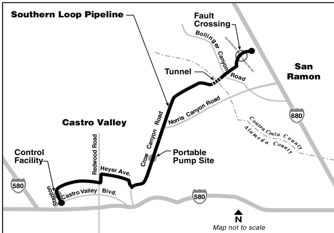
Figure 1. Southern Loop Pipeline, Showing Location of Calaveras Fault in San Ramon Area
