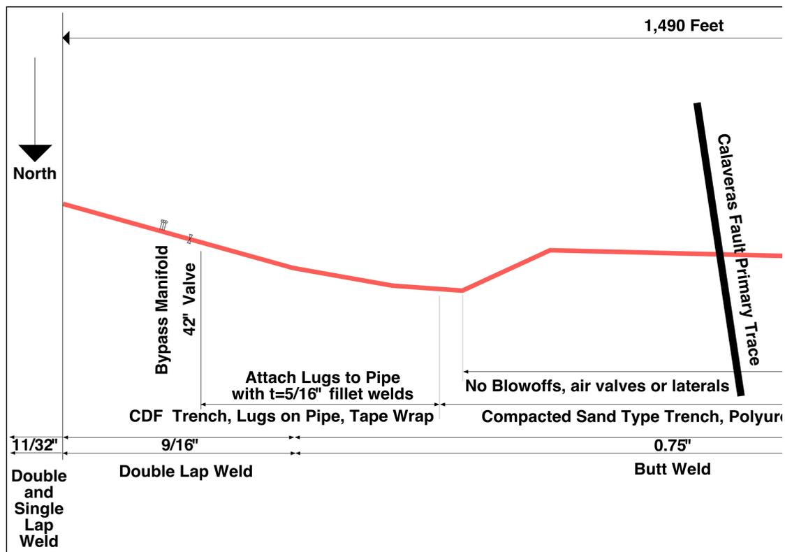
Figure 4a. Pipe Alignment With Main Design Features (East of Fault)
