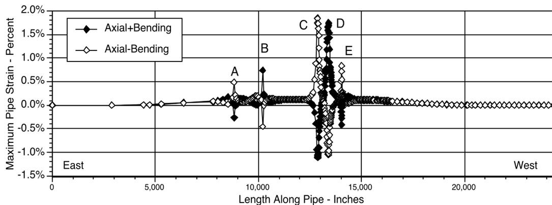
*Figure 5. Pipe Strains Due to Fault Offset*
