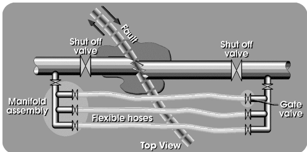
Figure 3. Bypass Design Concept
