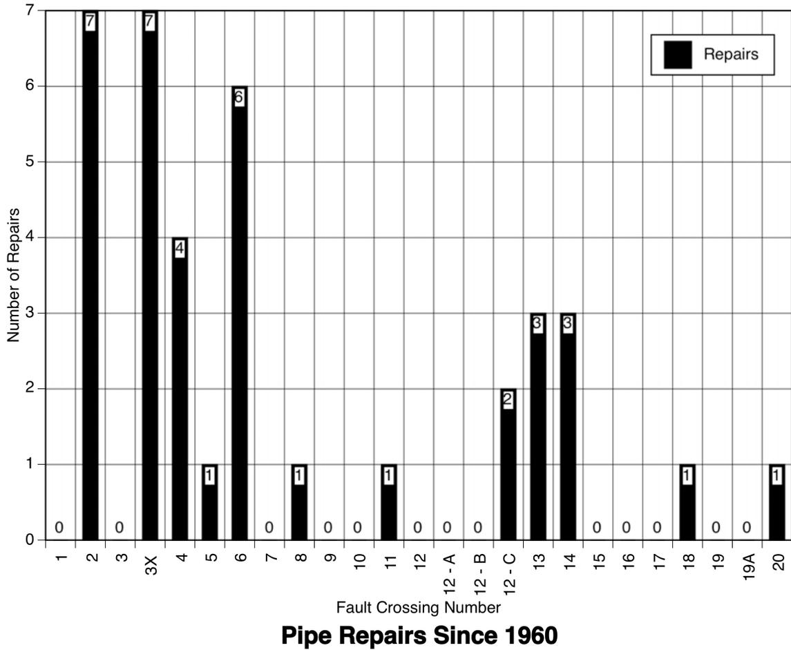
Figure 2. Leak history for twenty-five 20-inch and larger water pipes (EBMUD) due to ongoing Hayward fault creep, 1960-1990
