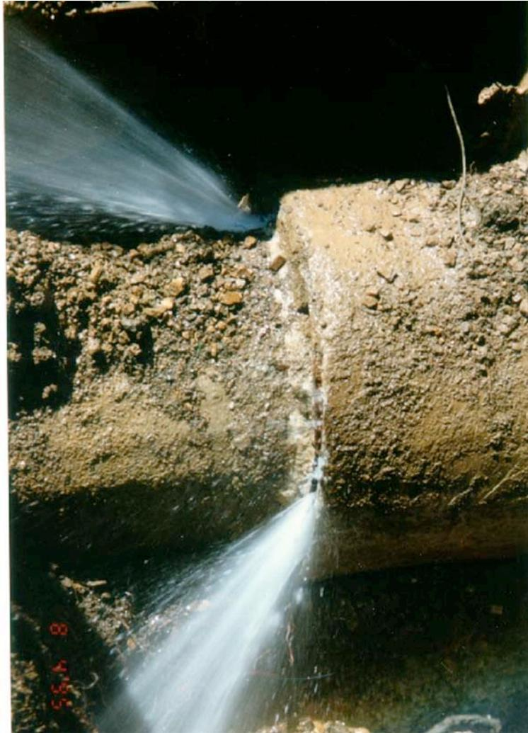
Figure 1. Leaking 30-inch diameter water pipe, damaged due to fault creep on the Hayward fault
