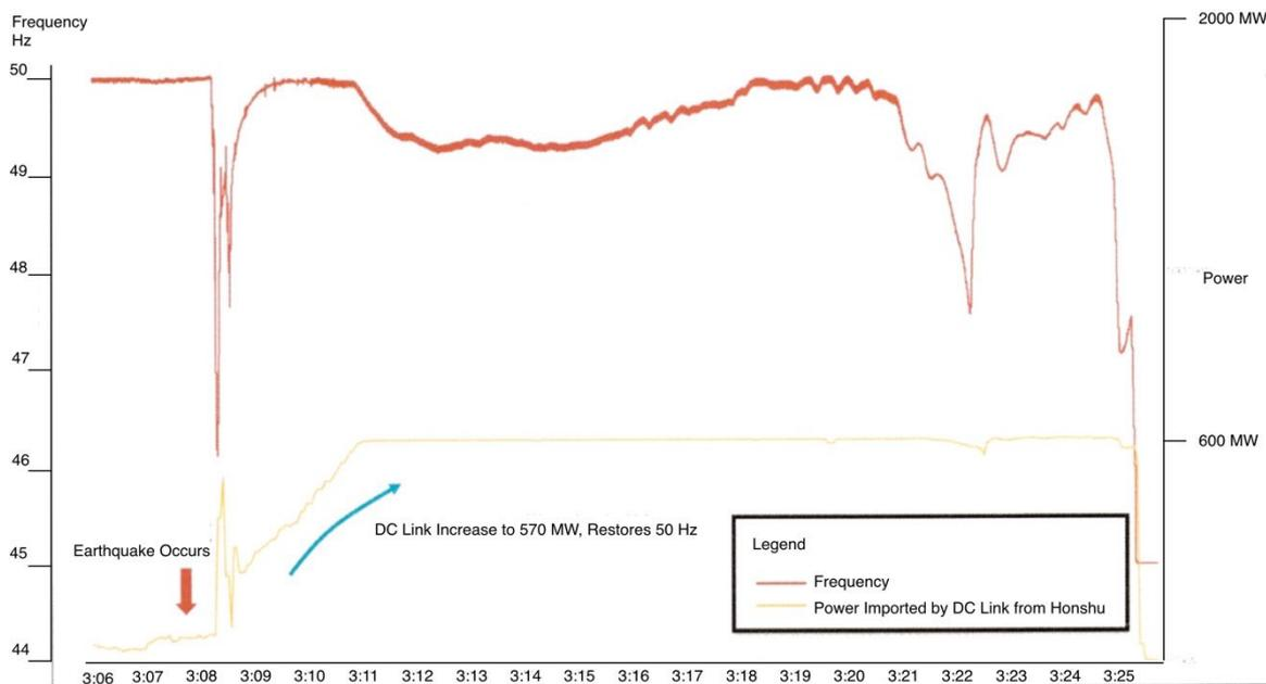
Fig. 5. System Frequency and DC Link Power Flow
