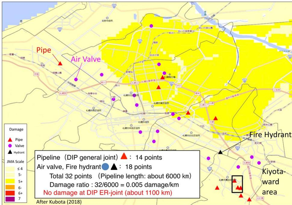
Fig. 9. Location of Water Pipeline Damage
