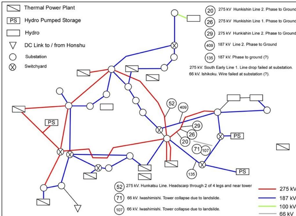
Fig. 7. Locations of Transmission Tower Damage
