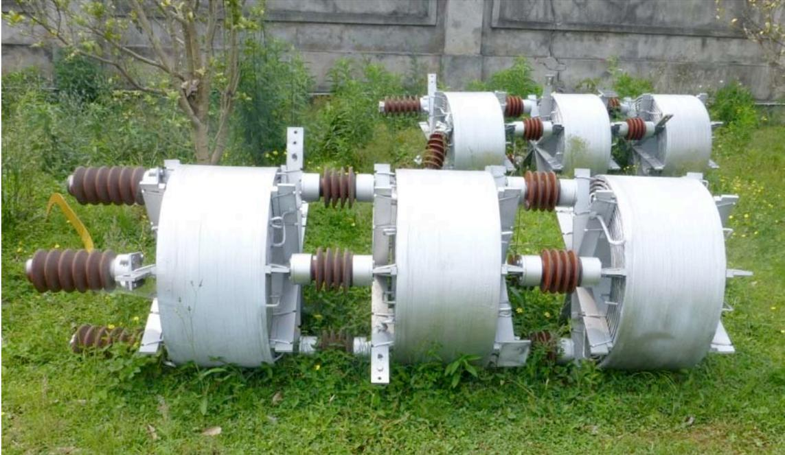
*Figure 4-12. Damaged Air Core Reactors*
