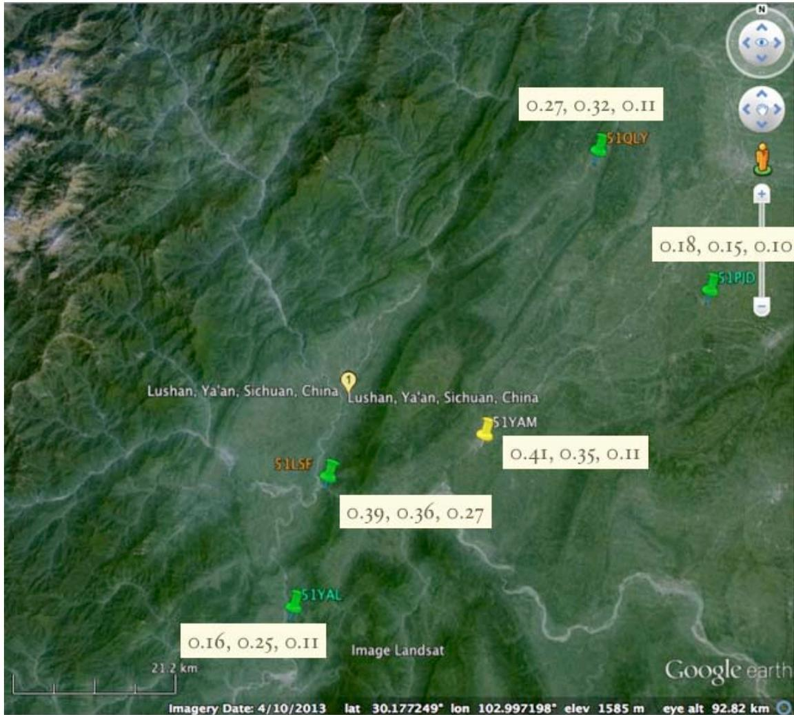
Figure 2-2. Recorded PGA Values (units in g, NS, EW, Vertical) (Base map copyright by Google)
