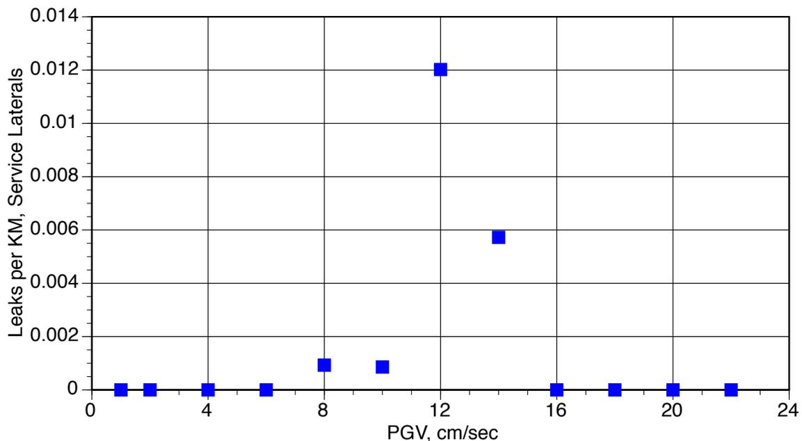
*Figure 17. Leak Rate for Service Laterals per KM*
