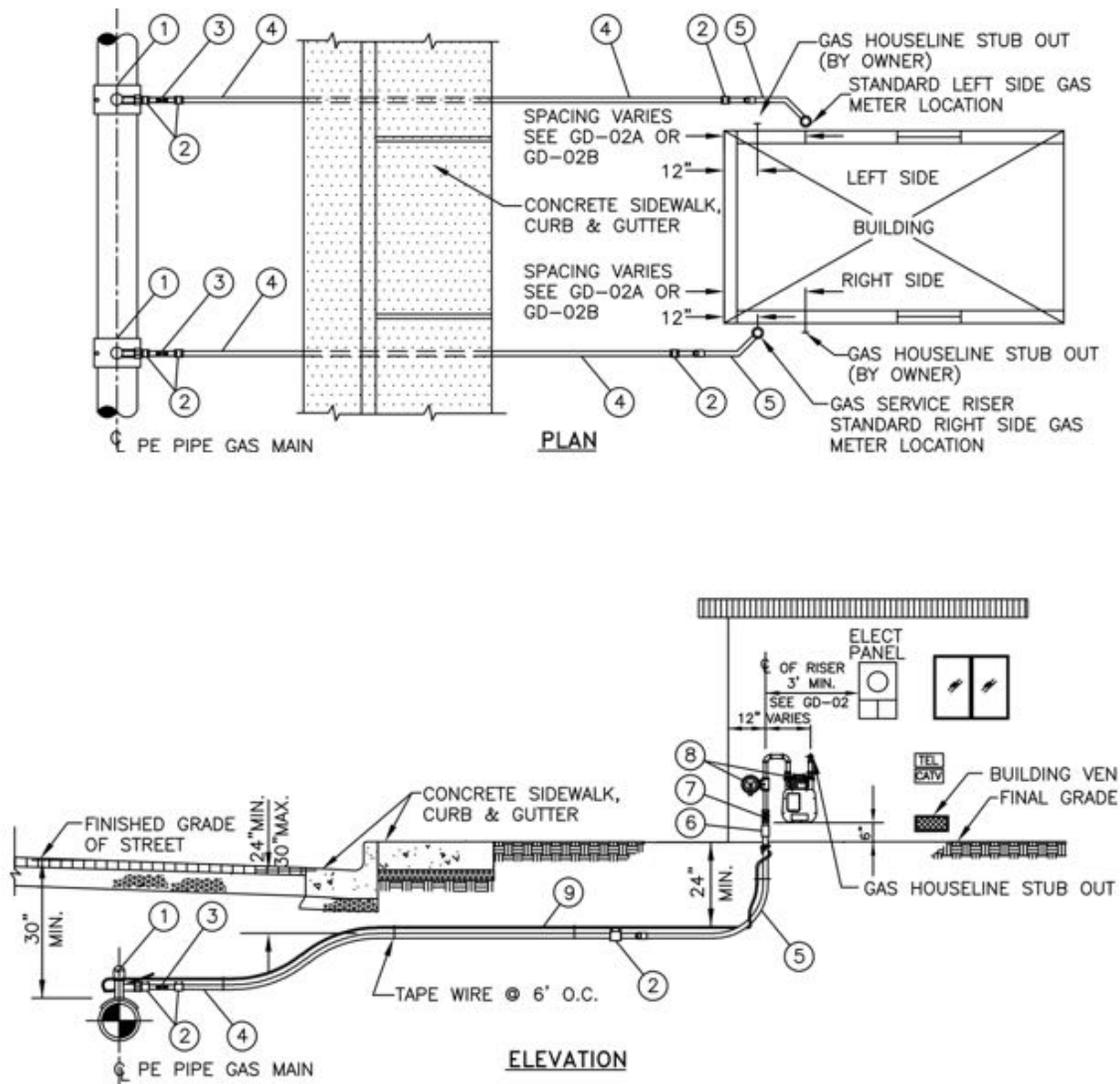
Figure 20. Typical Gas Service Line Details (see Table 5 for parts list)
