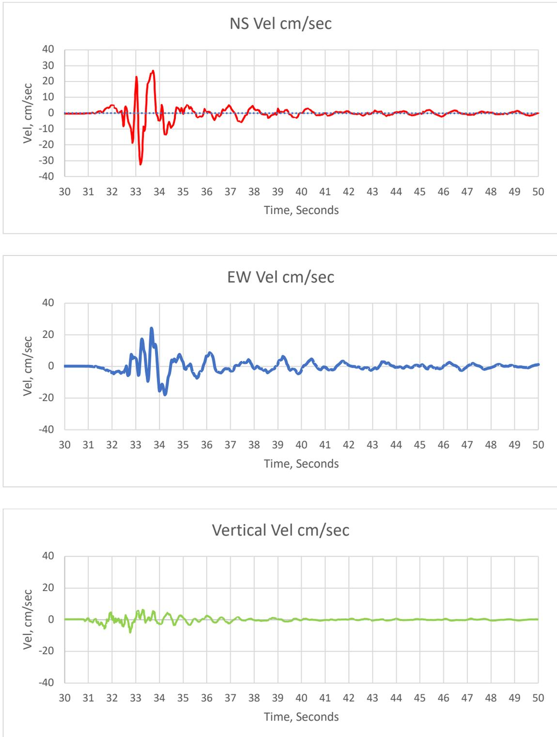
Figure 12. Ground Motions, Instrument LKC – Velocity Time Histories
