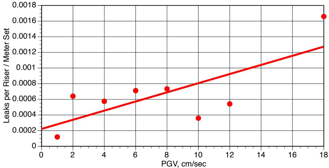
Figure 16. Leaks per Riser / Meter as a function of PGV
