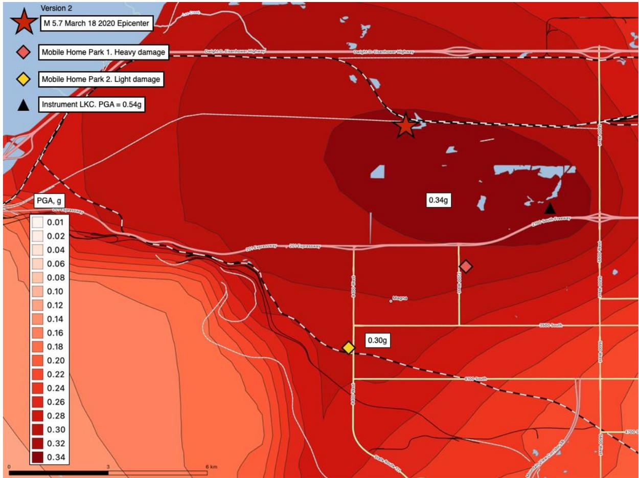
Figure 5. Magna Area Horizontal PGA Shaking Map (g) (Version 2 April 8 2020)
