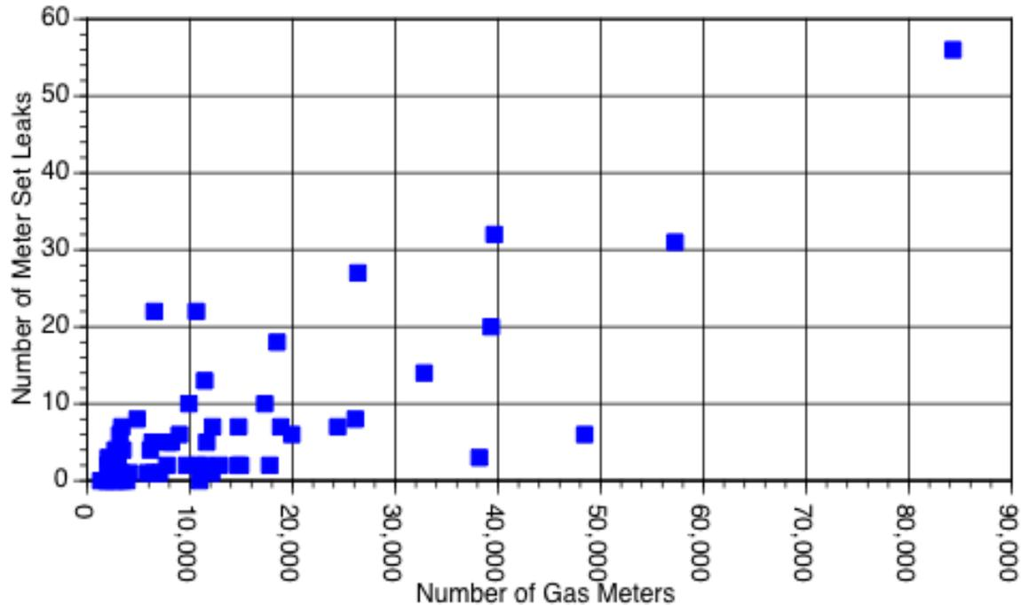
Figure 15. Number of Gas Meter Leaks vs Number of Gas Meters
