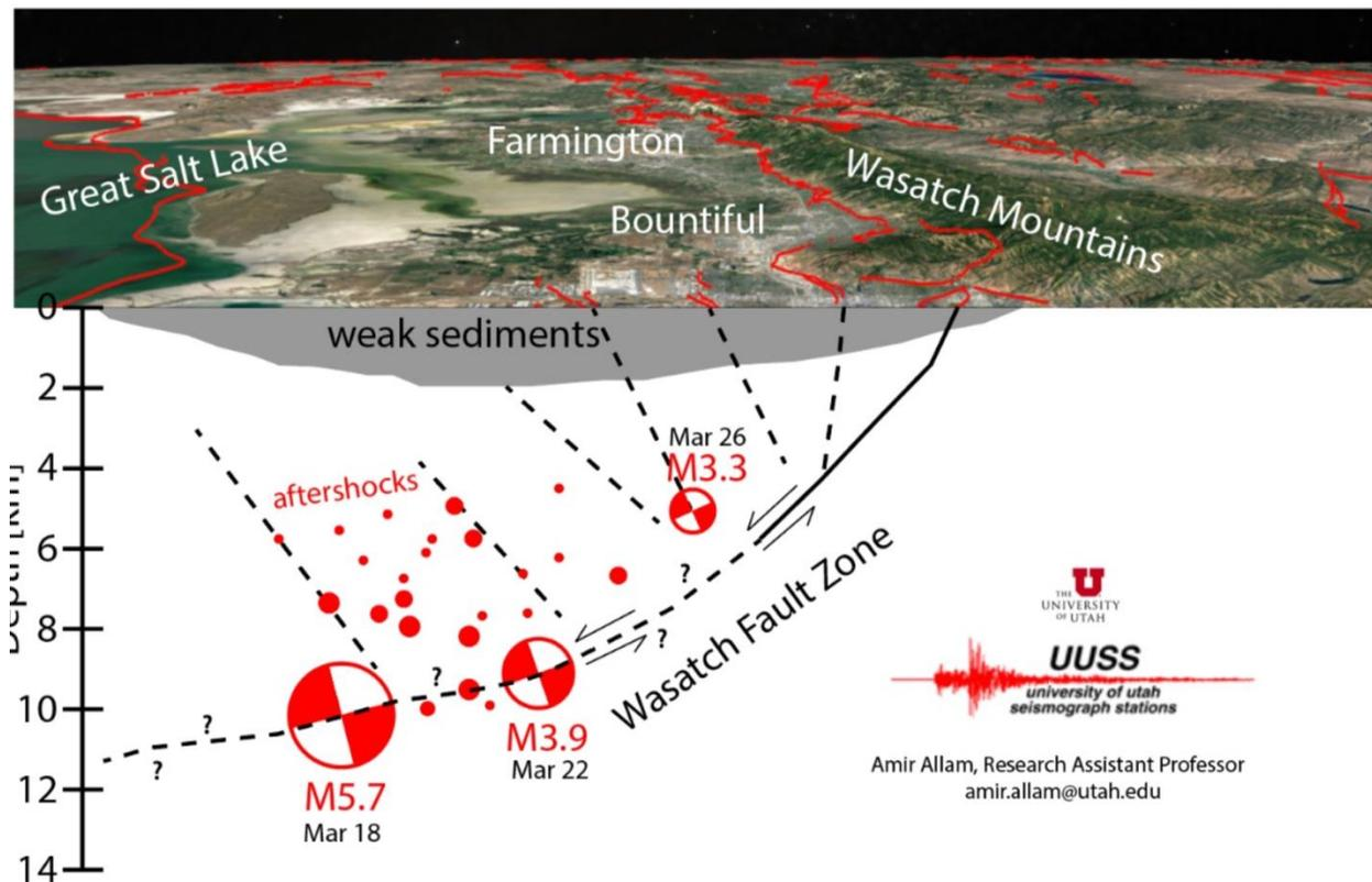
Figure 2. Cross Section showing Epicenter and Aftershocks (after UUSS)
