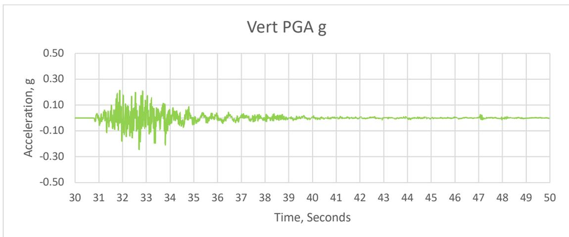
Figure 11. Ground Motions, Instrument LKC – Acceleration Time Histories
