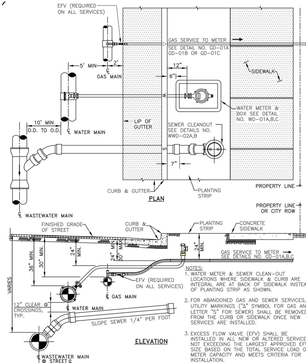
Figure 19. Typical Service Lateral Configurations
