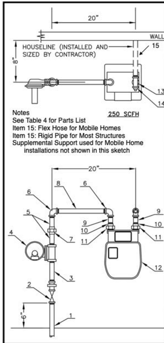
Figure 18. Common Riser and Gas Meter Typical Installation (see Table 4 for parts list)
