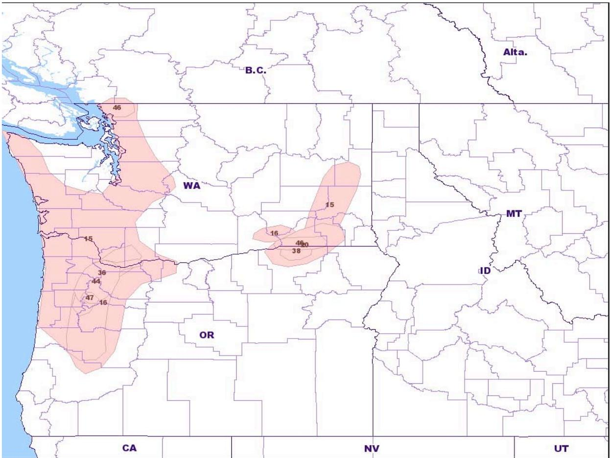
*Figure 4. Footprint of Ice Storms (shaded areas) in BPA Service Area, 1950 – 1959*
