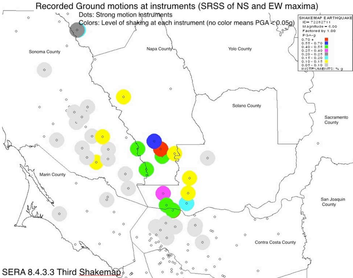
Figure 2-4. Strong Motion Instruments (version 3) (PGA)
