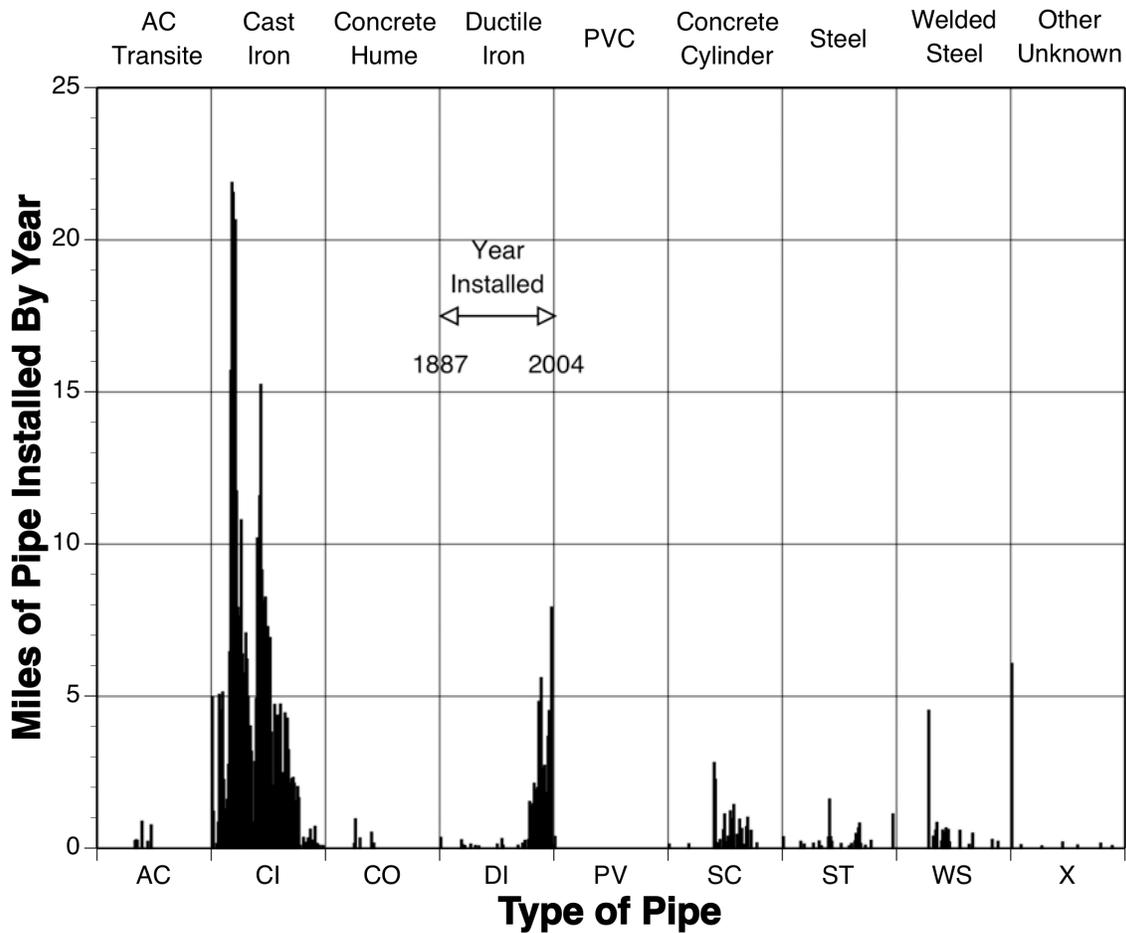
Figure 1. Pipes Installed, by Type and by Year
