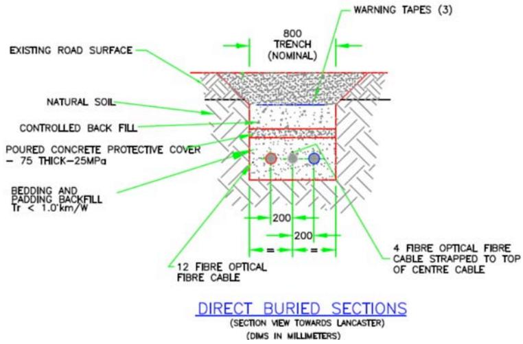
**Figure 9. Trench Design 66 kV XLPE-type Cable**
