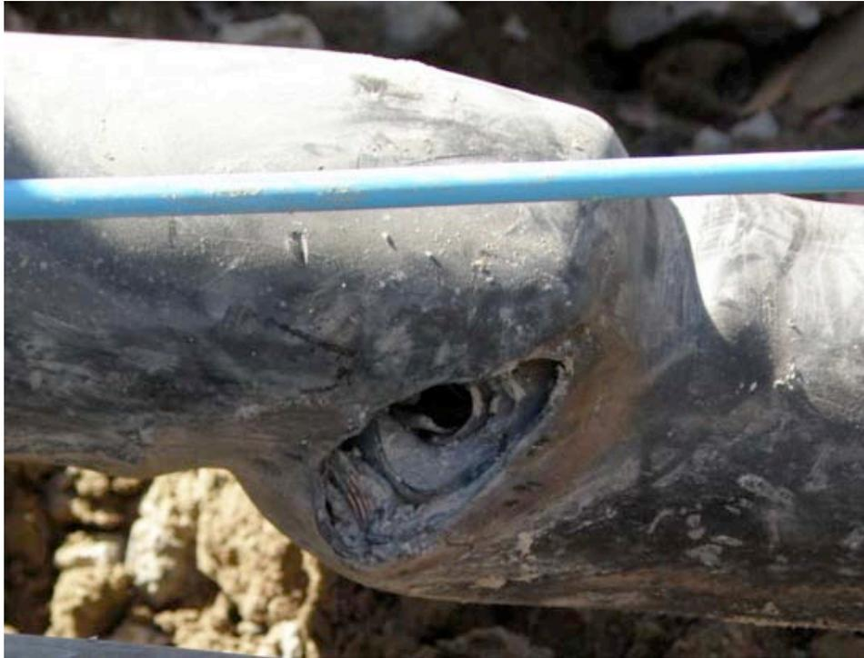
**Figure 12. Failed XLPE-Type Cable, Location 4**
