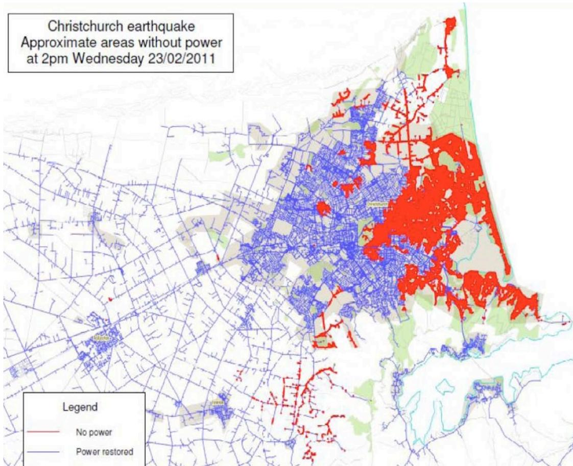
**Figure 2. Location of Power Outages, 24 hours Post-Earthquake**
