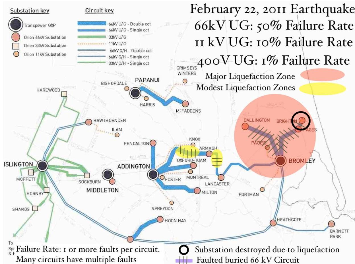
**Figure 1. Location of Orion 33 kV to 66 kV Distribution System and Liquefaction Zones**
