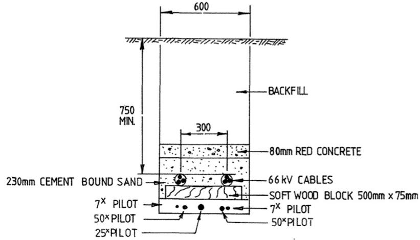
**Figure 5. Trench Design 66 kV Oil-type Cable**
