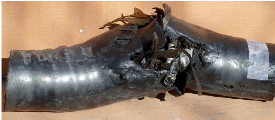
**Figure 8. Oil-Type Cable (Location 3)**
