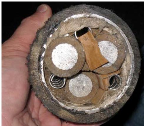
**Figure 7. Oil-Type Cable Cross Section**
