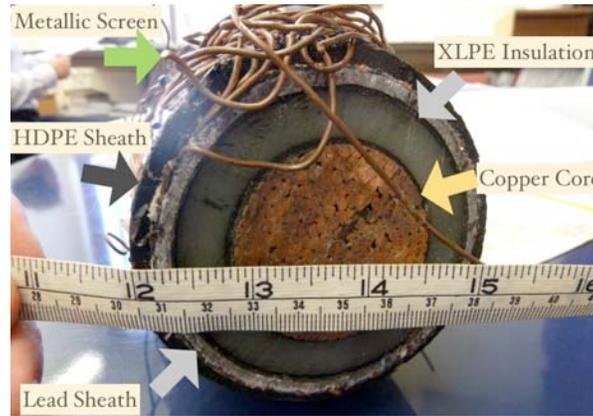
**Figure 10. Cross Section, XLPE-type Cable (Top scale in inches, bottom in cm)**
