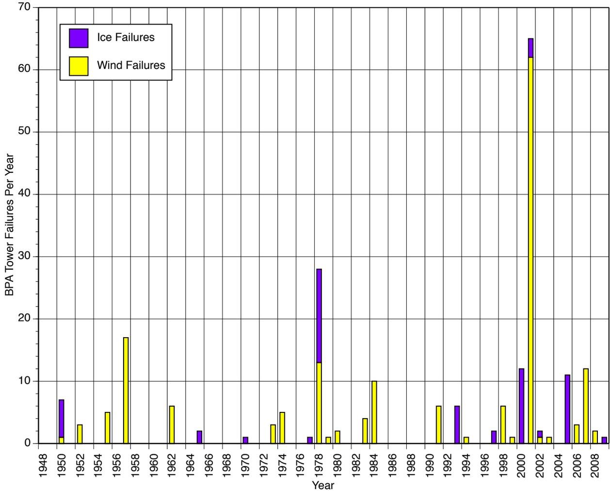
Figure 1. Transmission Tower Failures in Oregon, Washington and Idaho
