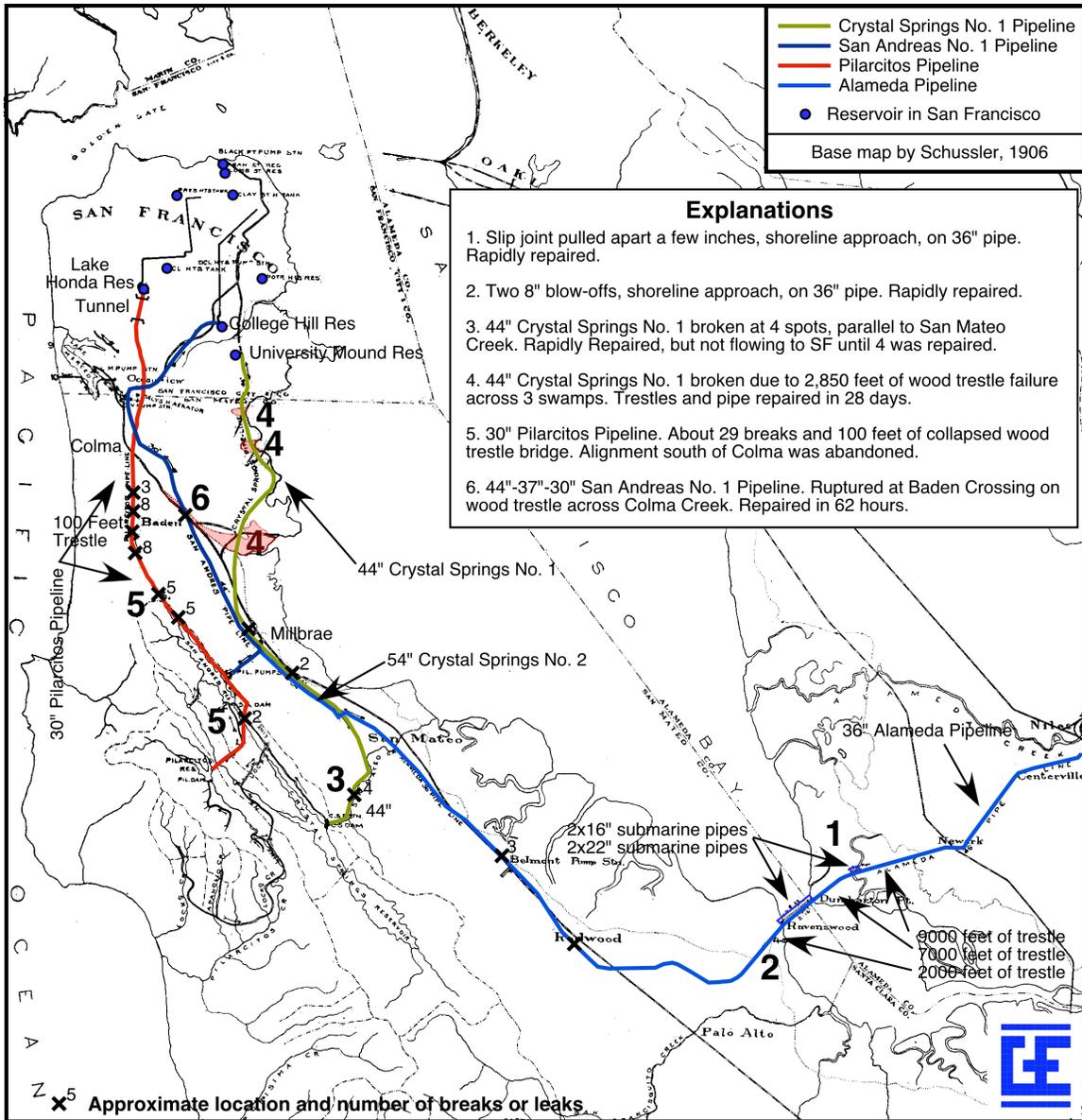
Figure 2. Damage to the SFPUC (Spring Valley Water Company) Transmission System, 1906
