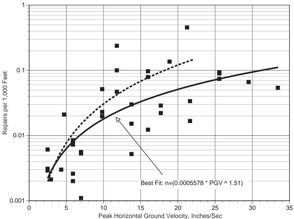
Fig. 5. Pipe Fragility Curve – Dashed Line Pre-Northridge, Solid Line Post-Northridge
