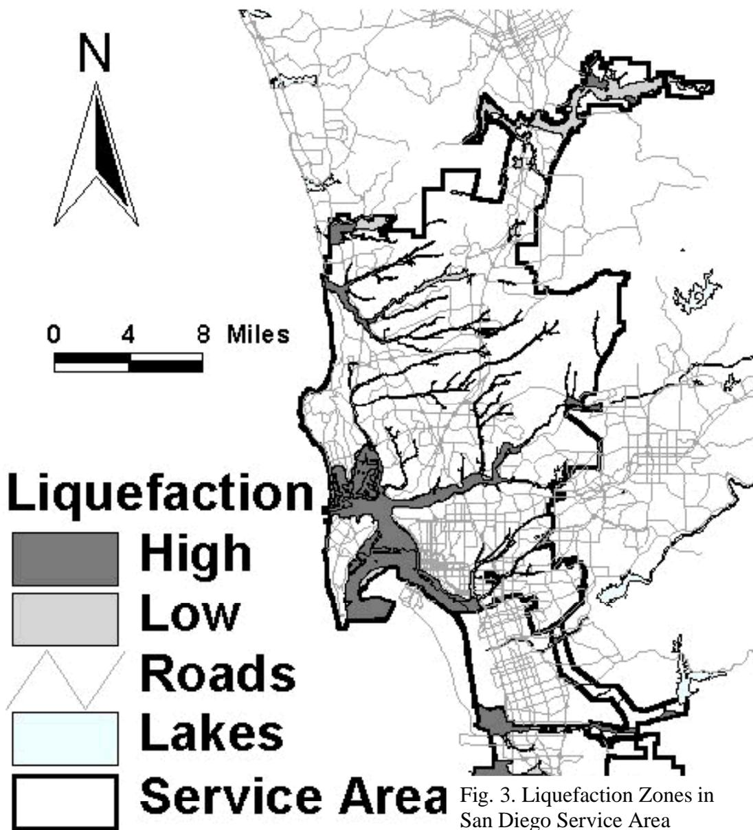
Fig. 3. Liquefaction Zones in San Diego Service Area
