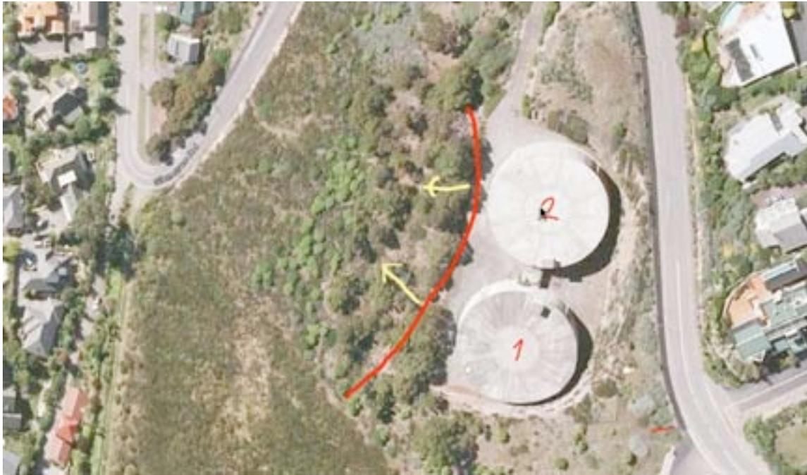
*Figure 6-21. Landslide Scarp, McCormacks Bay Tank Site*
