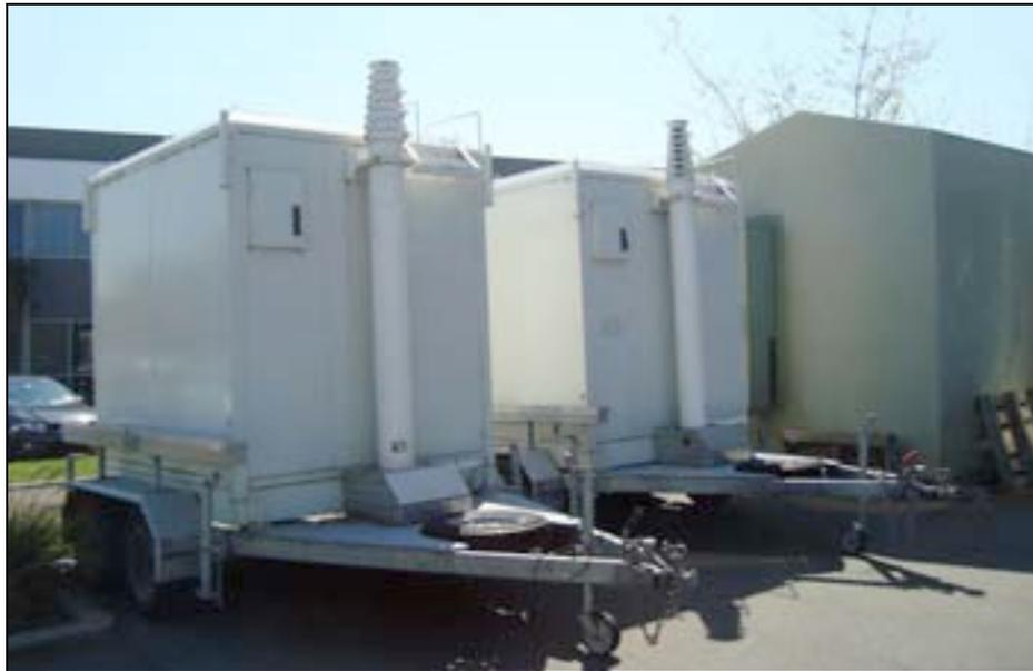
*Figure 5-5. Vodafone Cellsite On Wheels (COW).*
