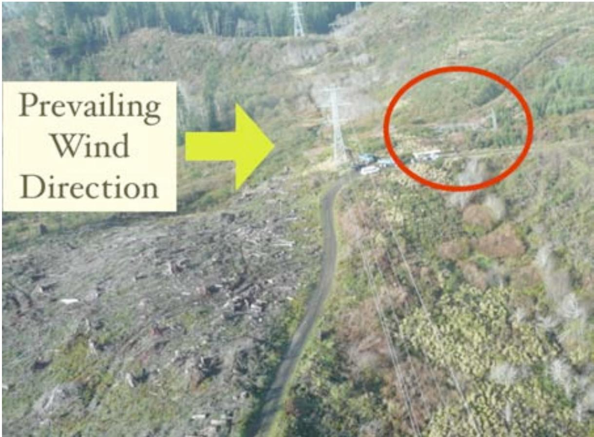
Figure 3. Case Study 1 Collapsed Tower Due to Wind Load
