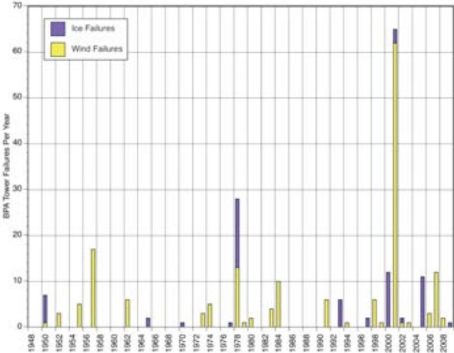
Figure 1 Reported Tower Failures (BPA), 1948 - 2009
