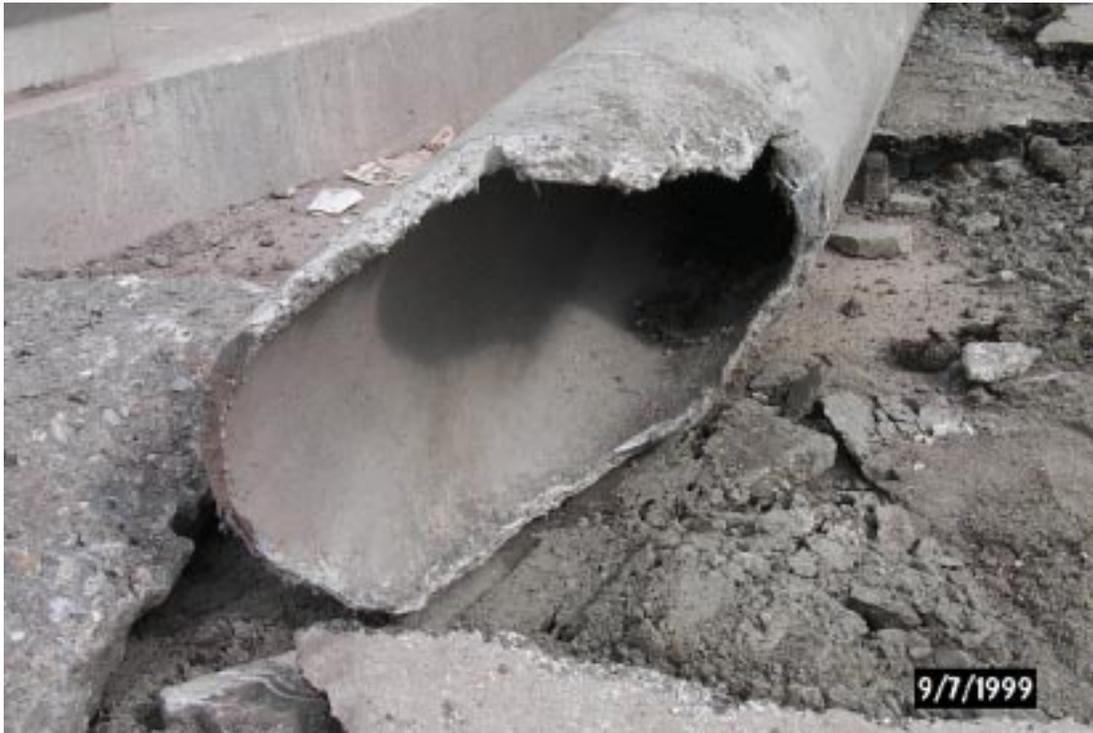
*Figure 12. Common Damage Pattern to AC Pipe In Areas with Settlement*
