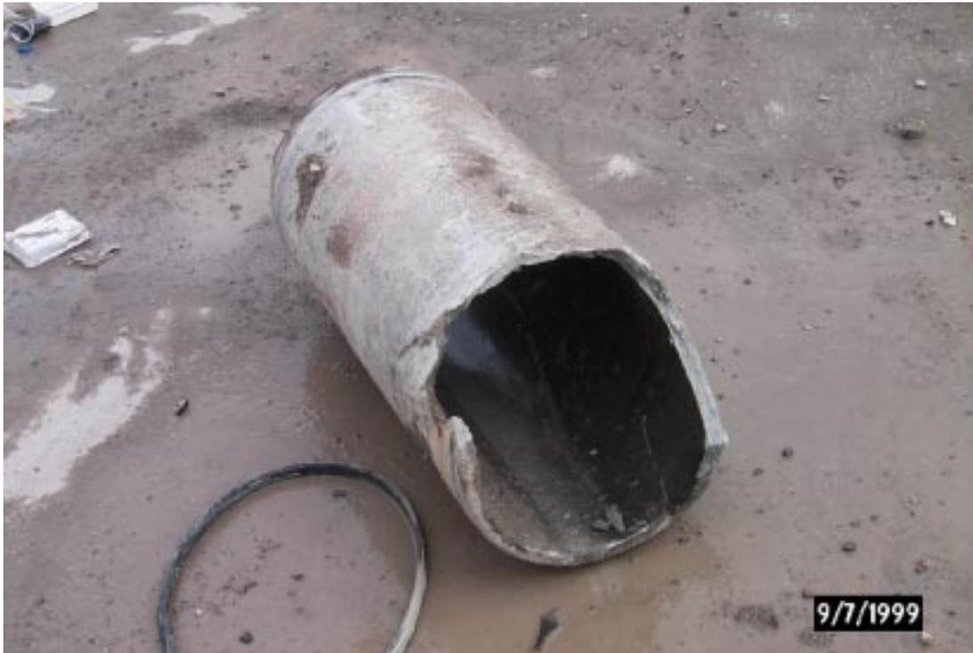
*Figure 11. Damage to 14" Diameter AC Pipe – Liquefaction Area*
