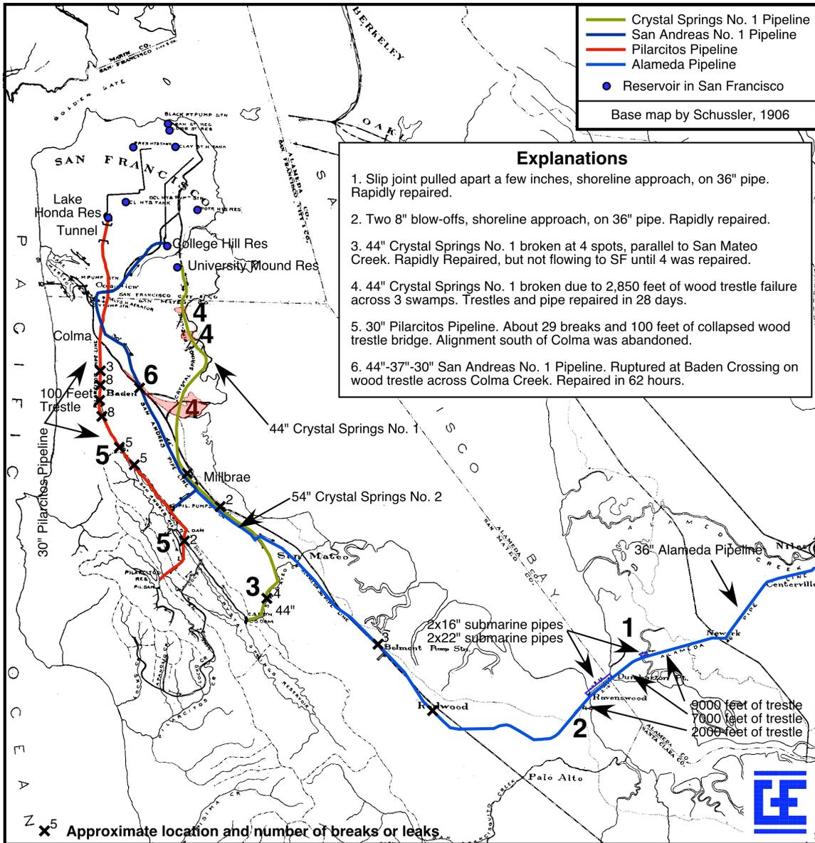
Figure 1. Damage to the SFPUC (Spring Valley Water Company) Transmission System, 1906
