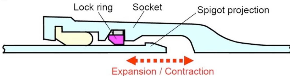
Figure 3-60. Chained Joint for Medium Diameter Ductile Iron Pipe
