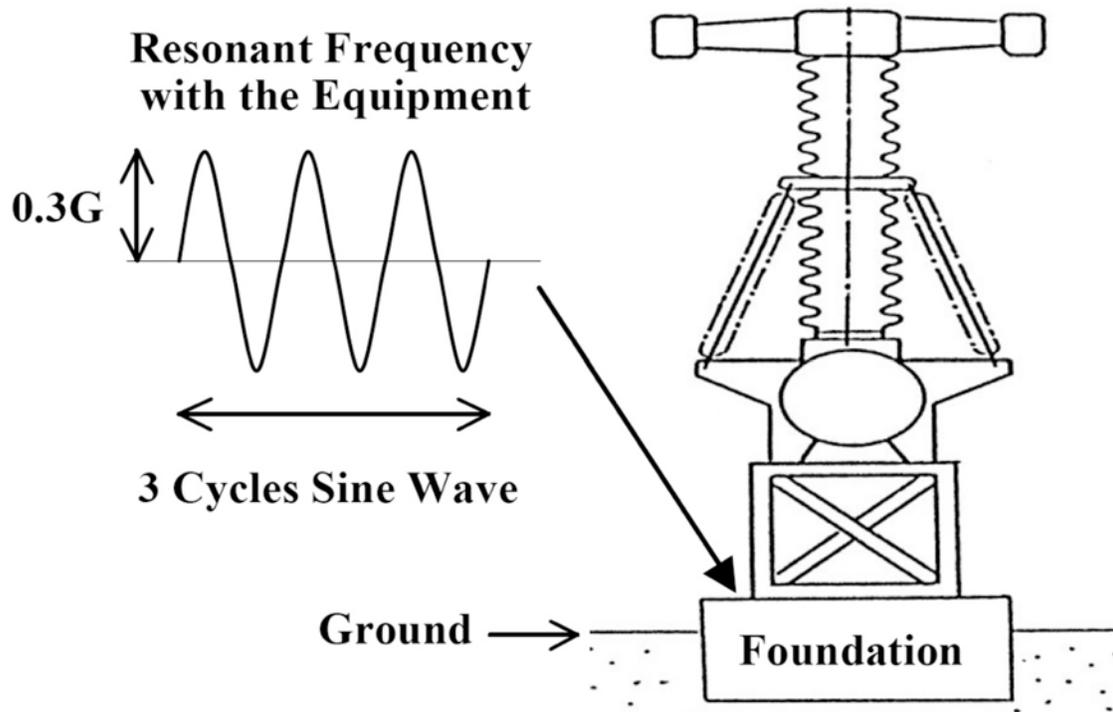
*Figure 4-2. Japanese Approach to Seismic Equipment Qualification at Substations*
