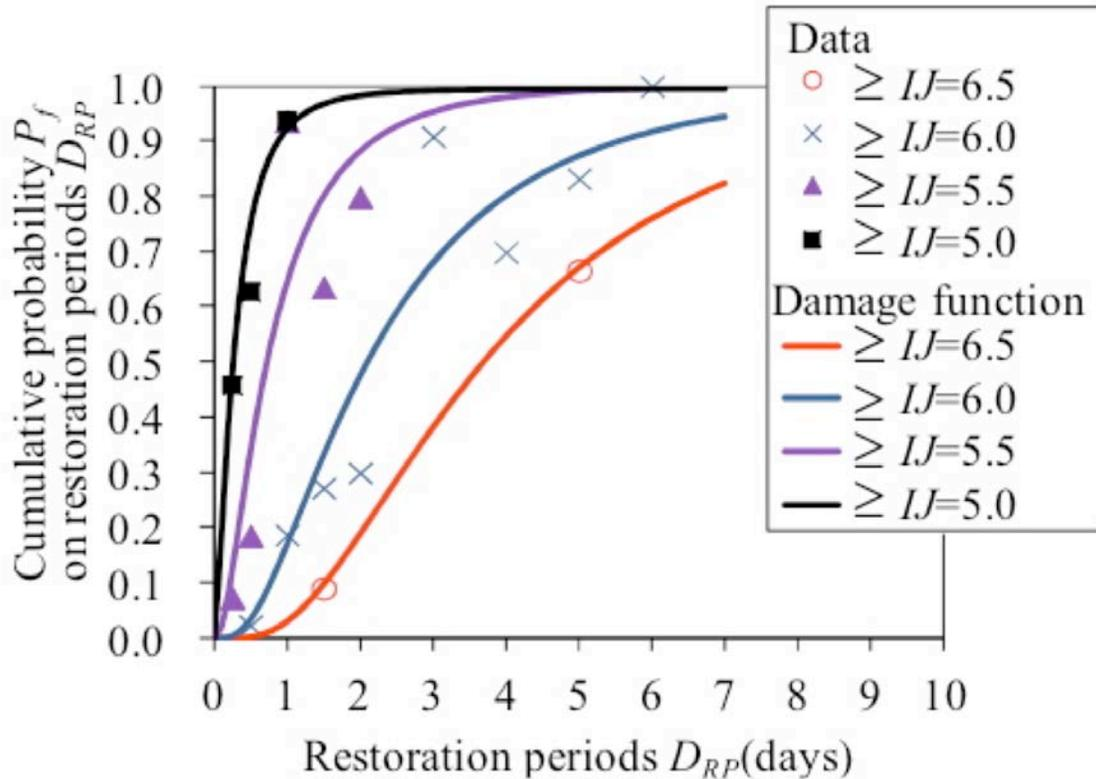
Figure 4-78. Fragility Curves for Duration of Power Outages Versus JMA Intensity, Near Tokyo
