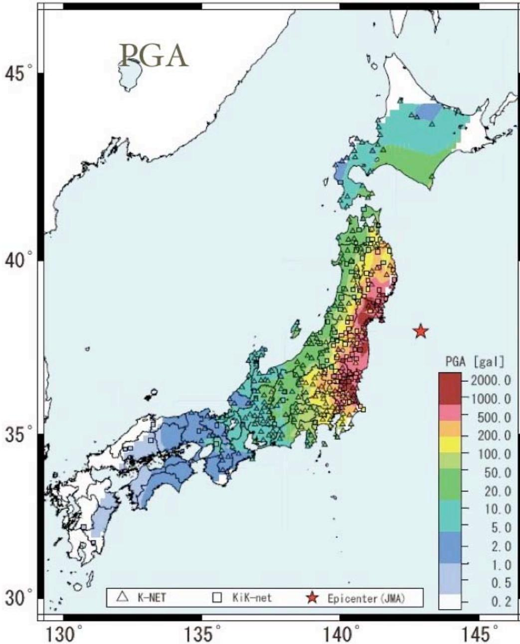
Figure 2-3. High Level Recorded PGA Values(Horizontal) in Regions of Japan
