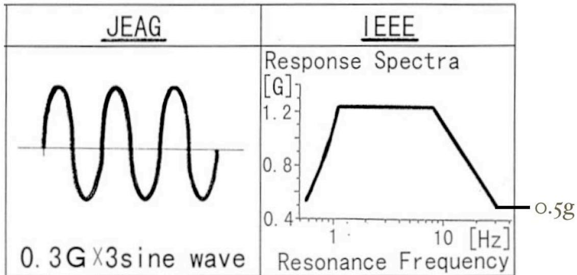
Figure 4-3. Comparison of Japanese and USA Approach to Seismic Qualification
