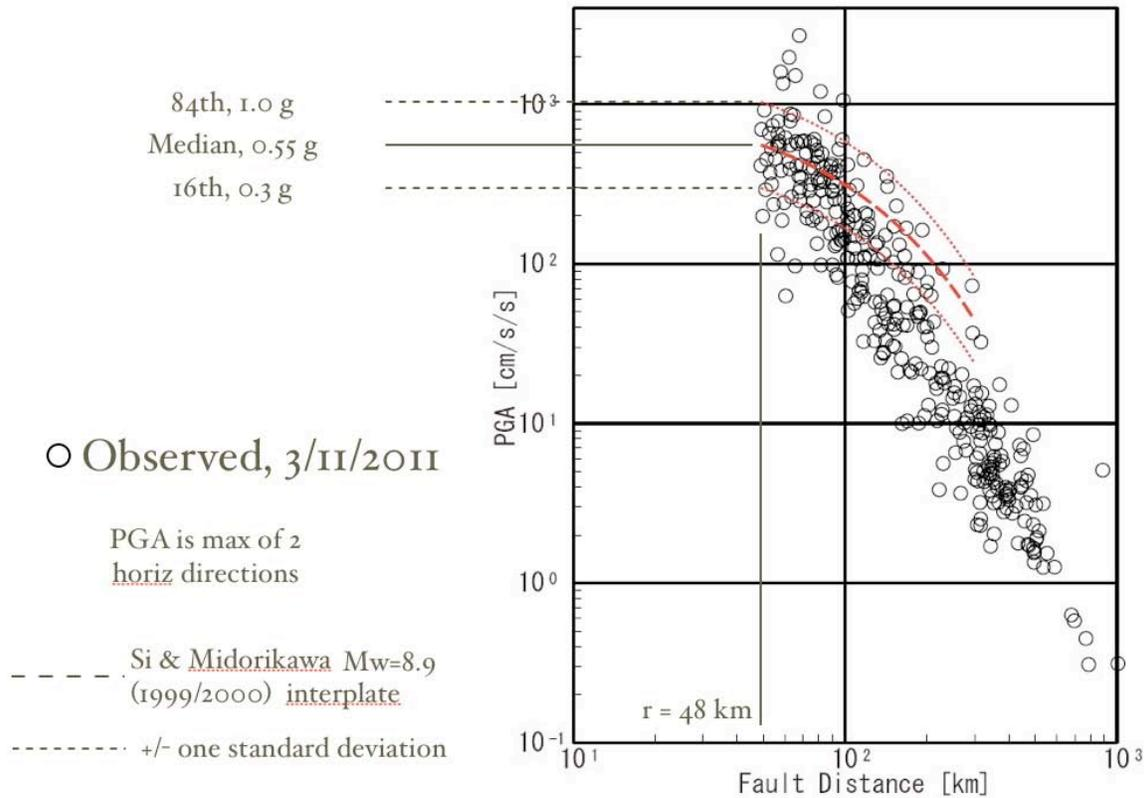
Figure 2-4. Attenuation of Ground Motion (PGA)
