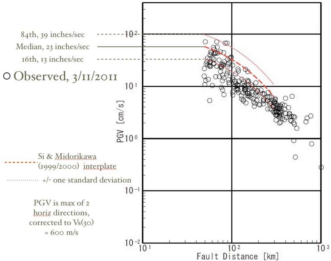
Figure 2-5. Attenuation of Ground Motion (PGV)
