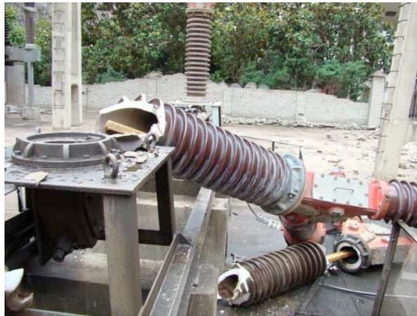
*Figure 2. Damaged Live Tank Circuit Breaker (110 kV)*
