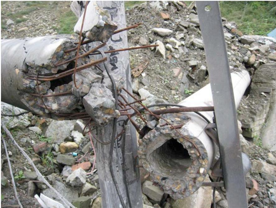
*Figure 12. Collapsed 10 kV Distribution Pole (10 inch diameter, 2.5-inch wall thickness)*
