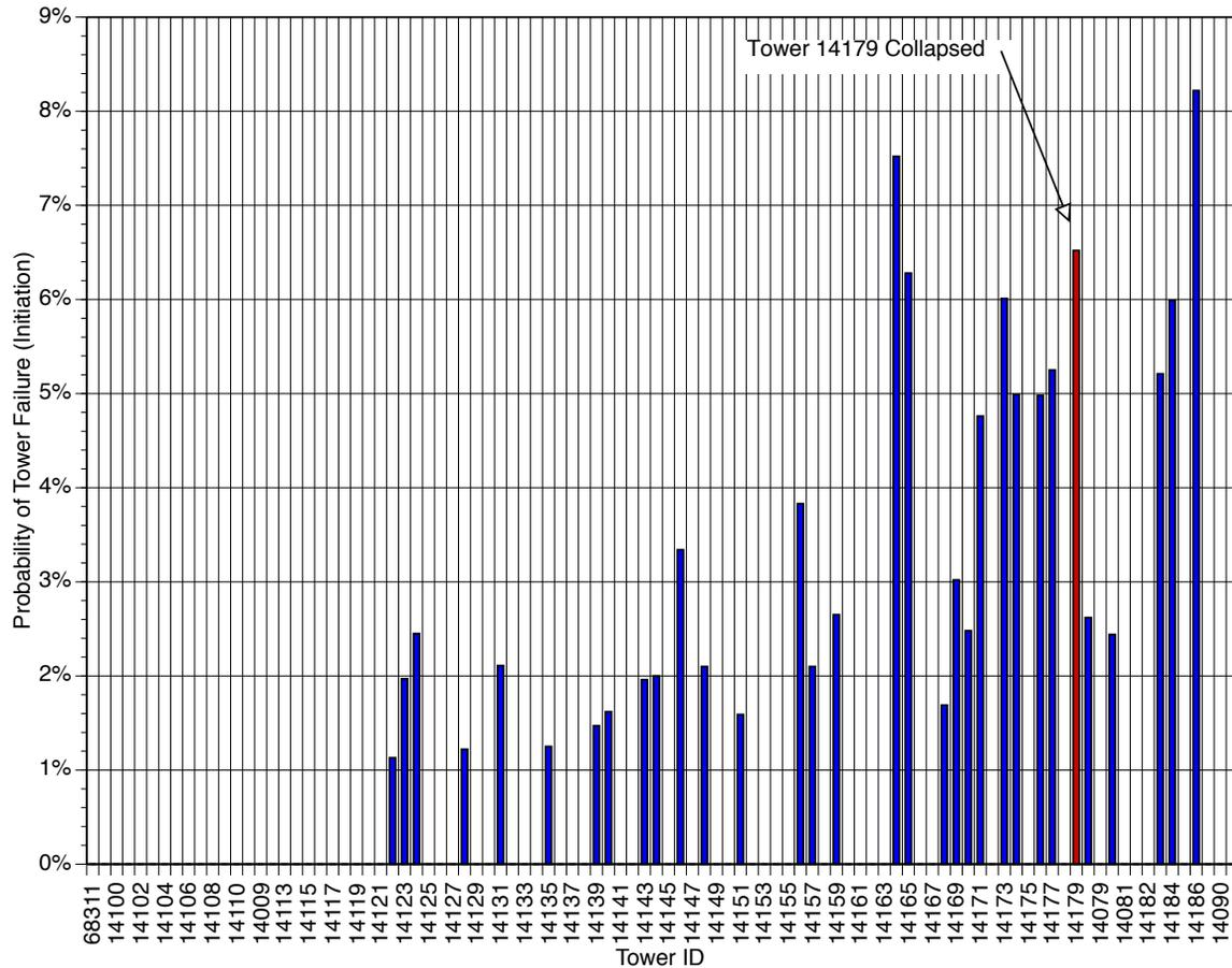
**Figure 3-11. Case 1. Satsop-Aberdeen Tower Failure Probabilities**
