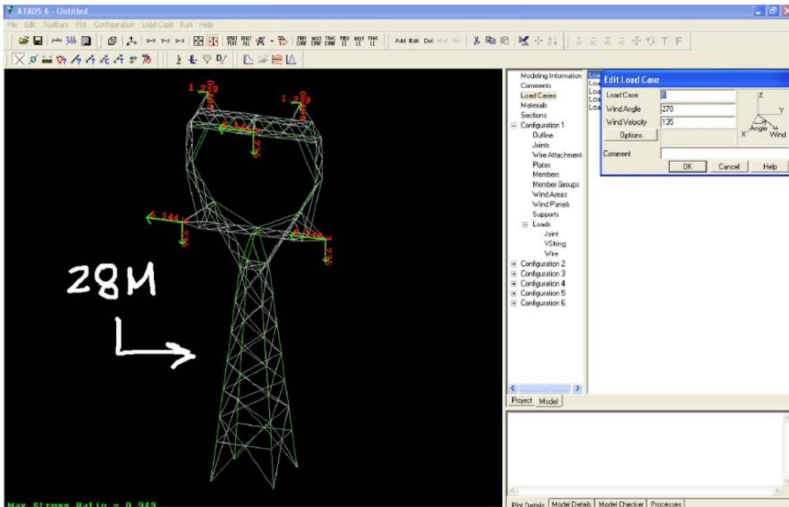
Figure 4-9. ATADS Model of 28M1 Tower
