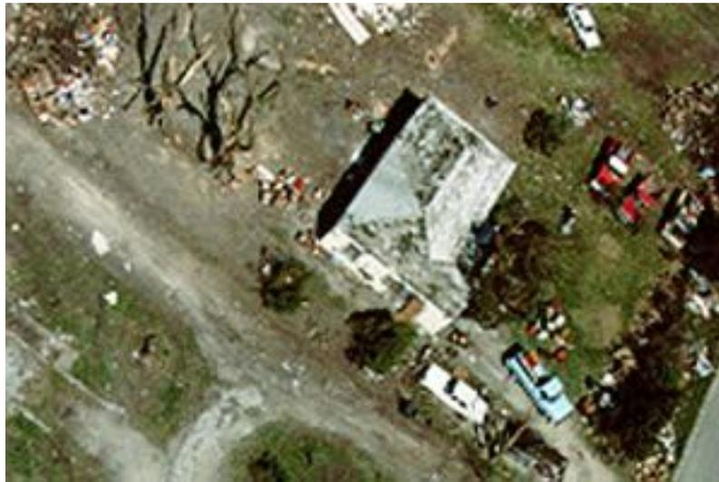
Figure D-1. Typical F0 Tornado Damage. Note the trees are stripped of leaves, but the trees remain standing. Only light roof damage and a few missing shingles.
