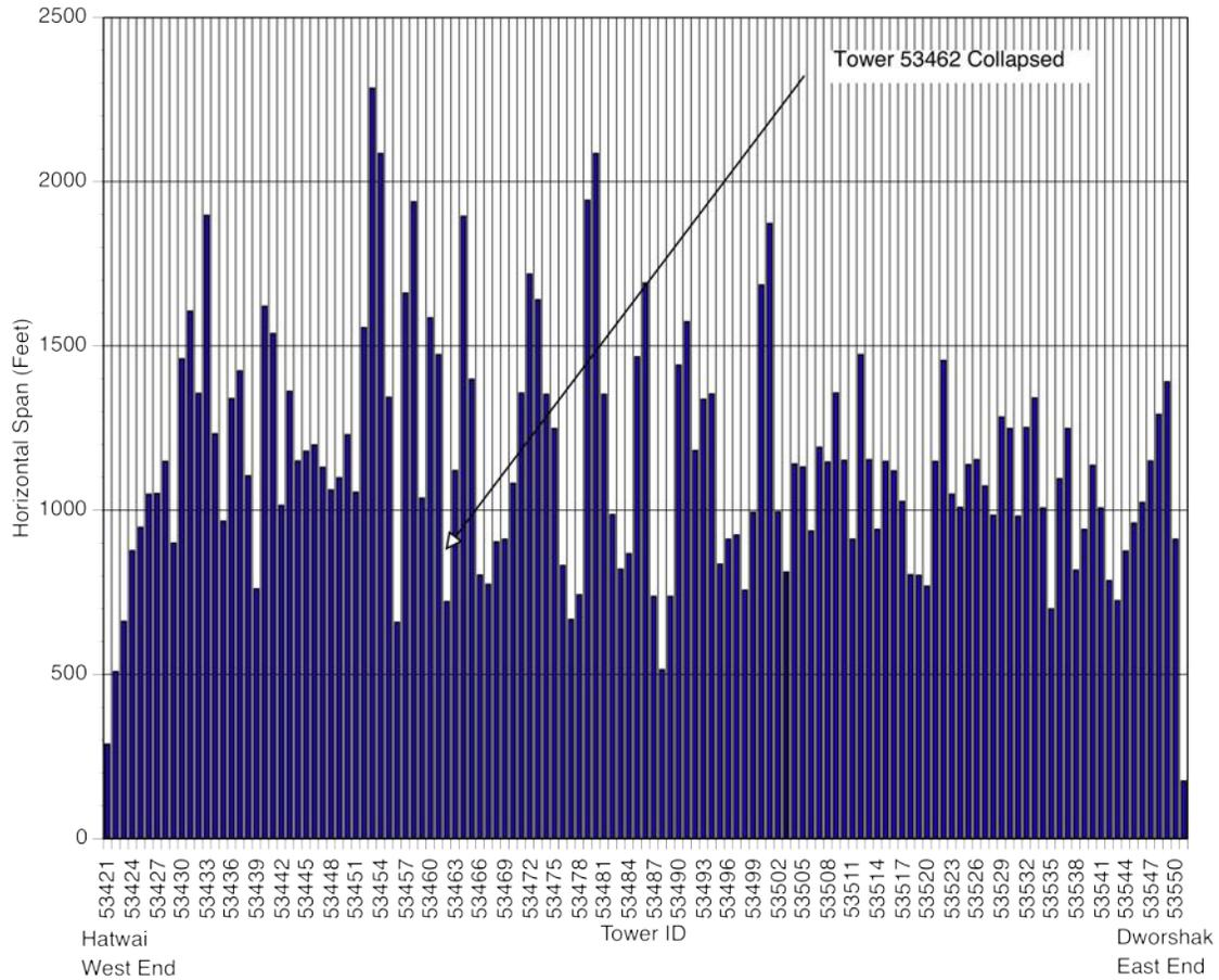
Figure 4-14. Horizontal Spans, Hatwai – Dworshak
