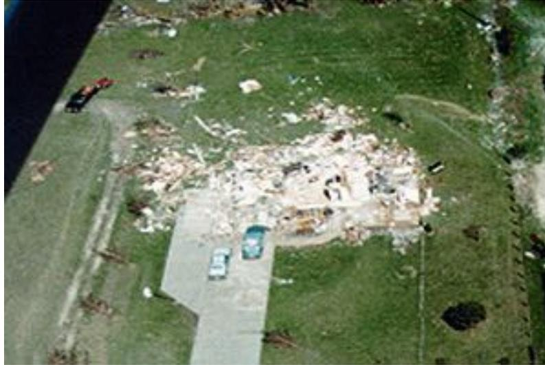
Figure D-5. Typical F4 Tornado Damage. This home is almost completely obliterated, with no walls standing. The debris from the home is where the house once stood.
