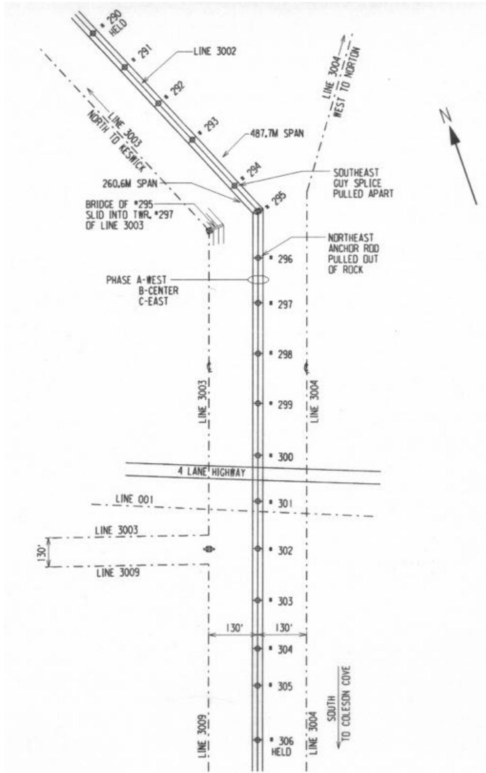
Figure 5-1. Line 3002 – Plan (Not to scale)
