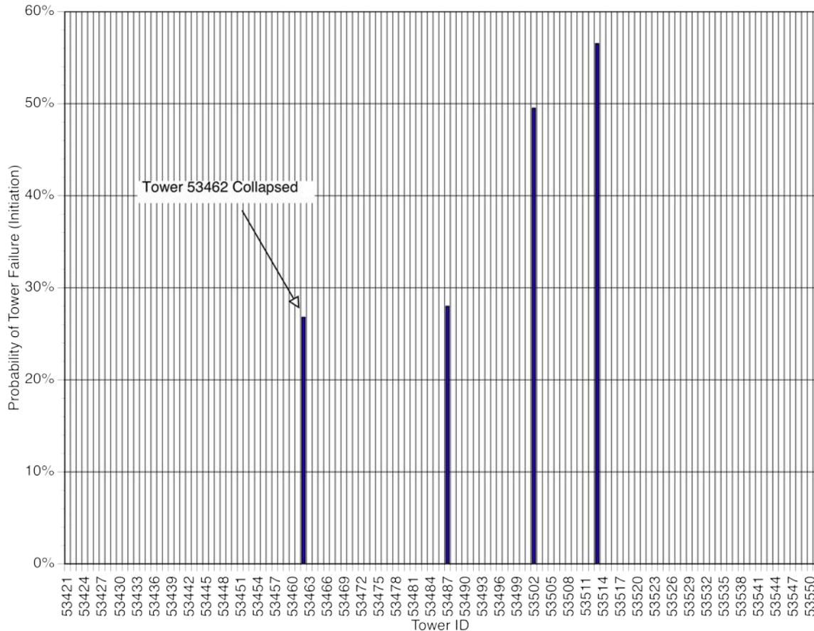
**Figure 4-16. Tower Initiation Failure Rates, Hatwai – Dworshak**
