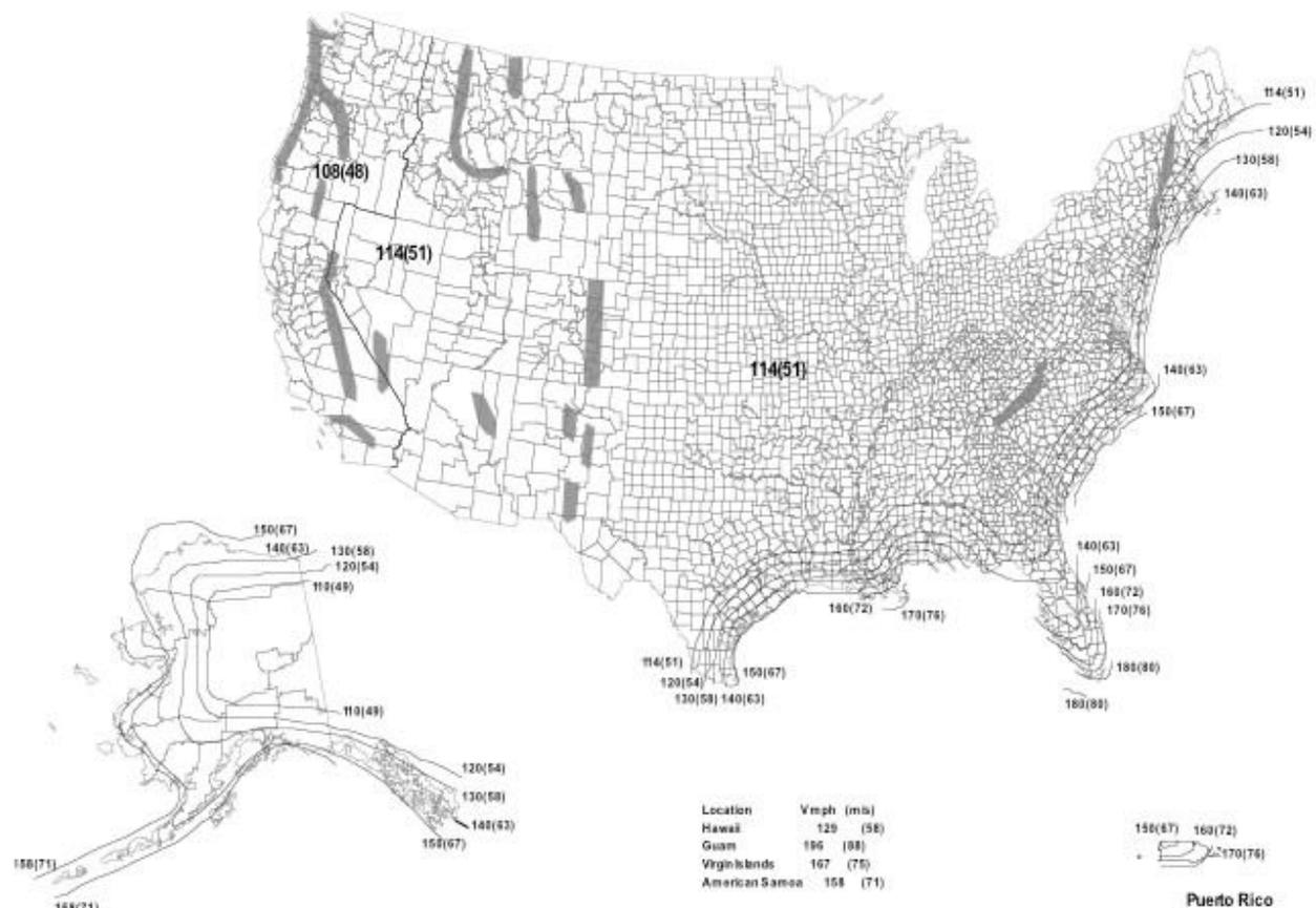
Figure A-4: USA: ASCE 7-10 Wind Map (mph, m/s) 700 Year RP
