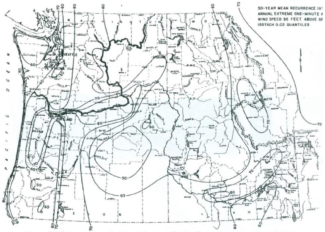
Figure A-6: PNW: BPA Wind Map, 1980 (50 Yr, mph, at height Z = 30 feet, One Minute)
