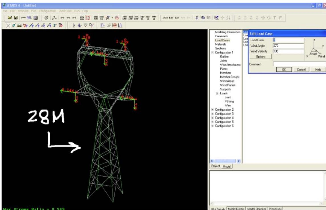
Figure 4-9. ATADS Model of 28M1 Tower
