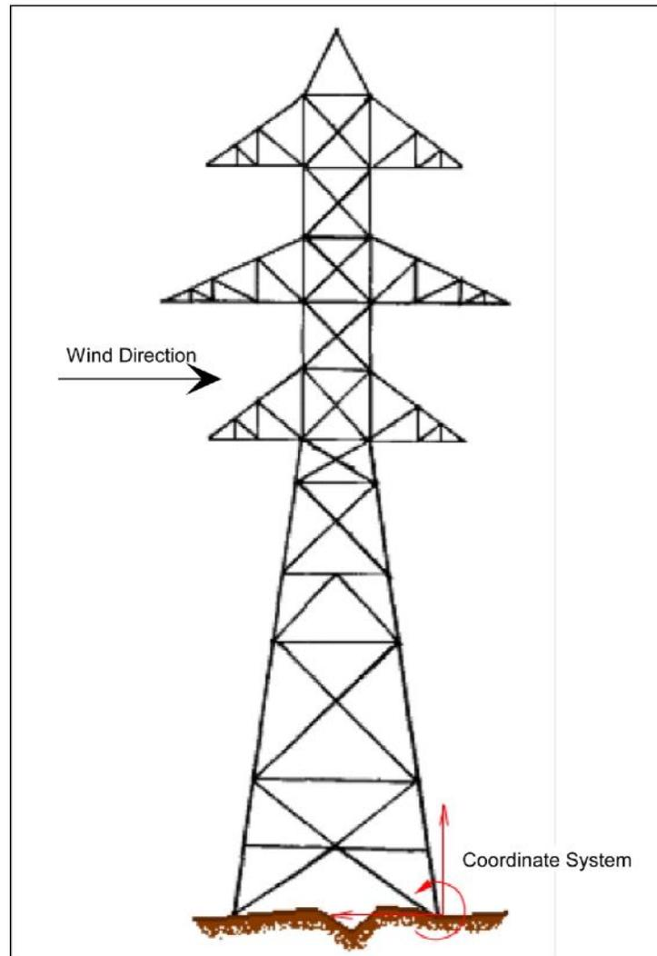
**Figure 3-10 Generic Tower Coordinate System**
