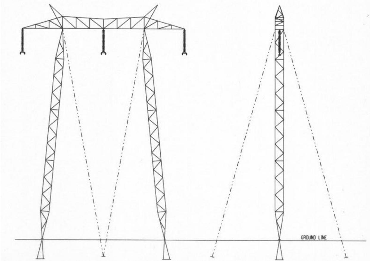
Figure 5-4. Structure 291-294, 296-305 (Guyed Tangent Towers)
