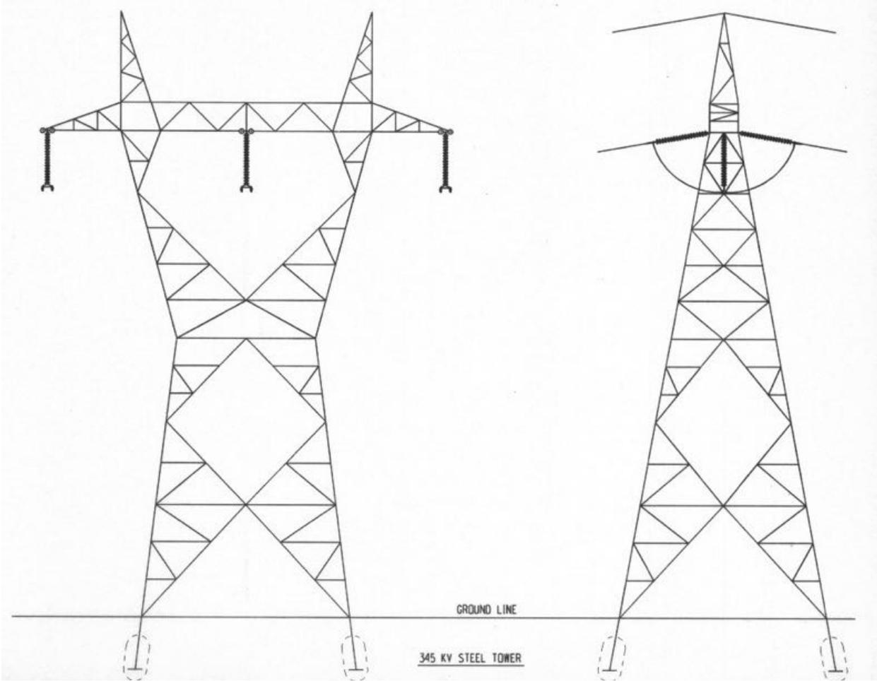
Figure 5-3. Structure 295 (Dead End Tower)
