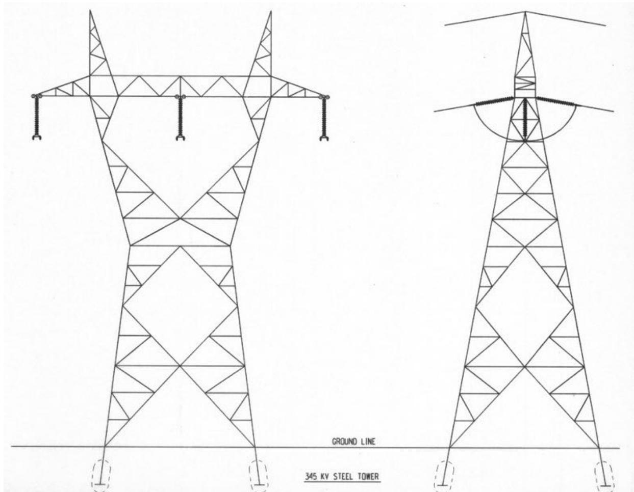
Figure 5-3. Structure 295 (Dead End Tower)
