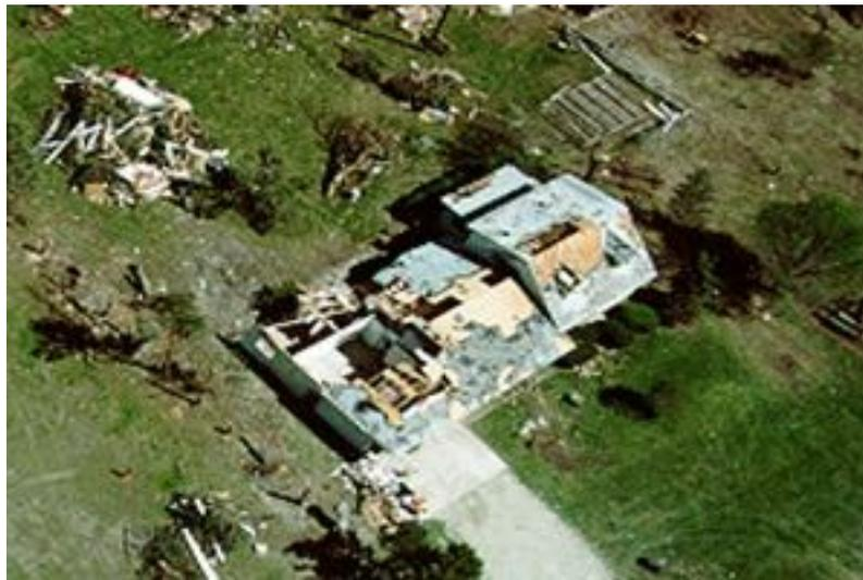
Figure D-2. Typical F1 Tornado Damage. Note the uprooted trees and missing shingles from the roof. There is significant roof damage.
