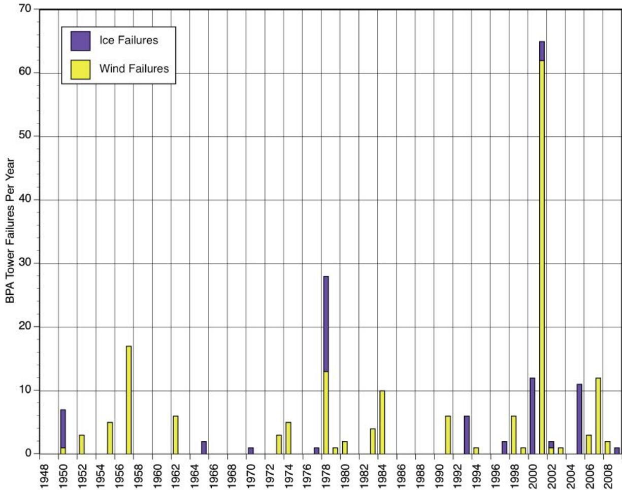
Figure 3-1 Reported Tower Failures (BPA), 1948 - 2009
