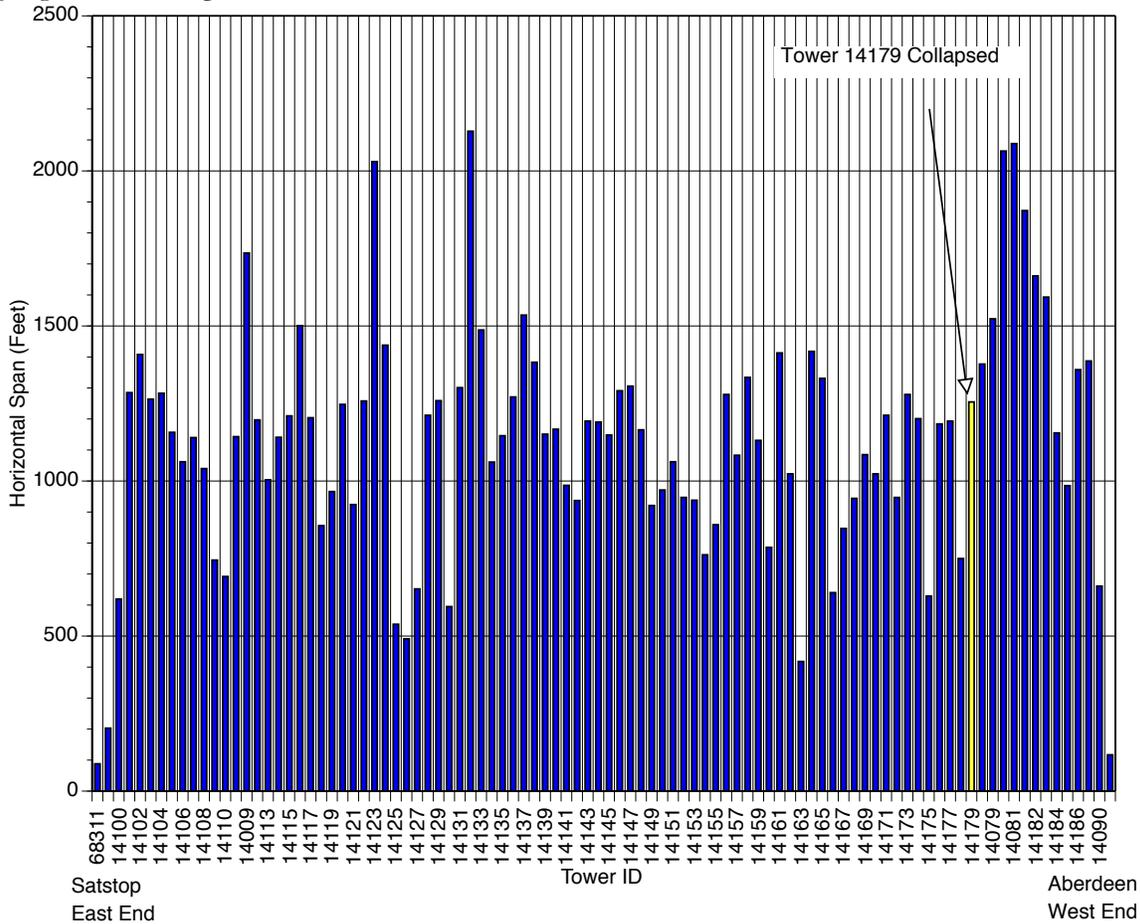
**Figure 3-8 Satsop-Aberdeen Circuit Spans**
