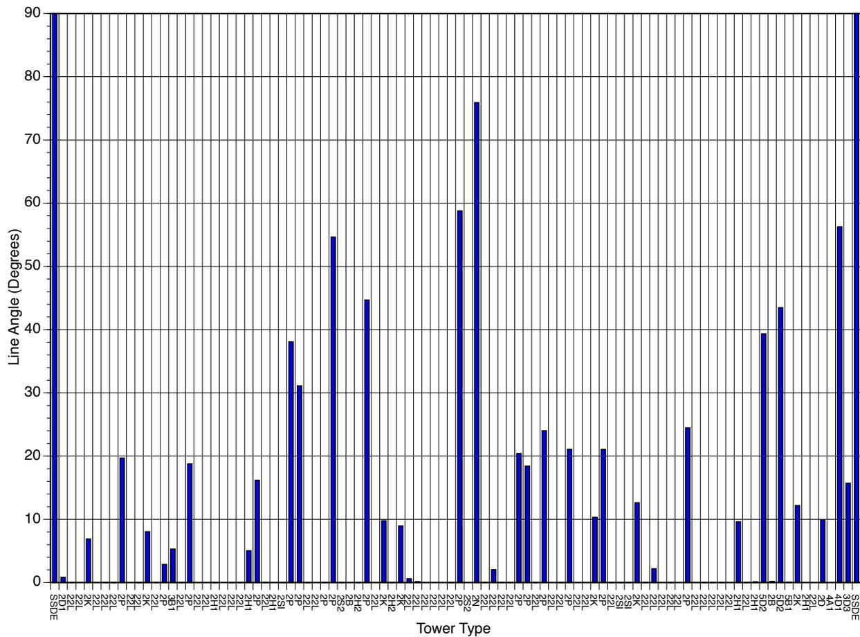
Figure 3-9 Satsop-Aberdeen Tower Types and Line Angles
